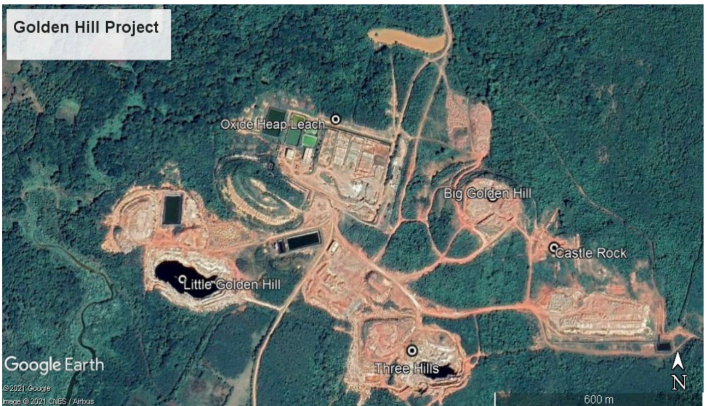
Mined oxide deposits at Golden Hills underlaid by an outcropping interconnected sulphide deposit
