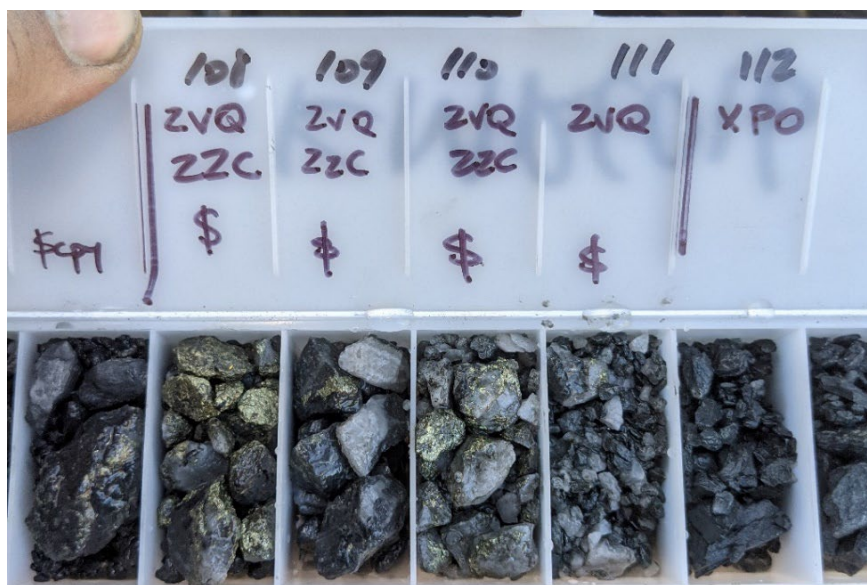
Figure 5: KMRC016 chip tray showing significant chalcopyrite-quartz veining from 106-111m downhole at Grant’s Find.
