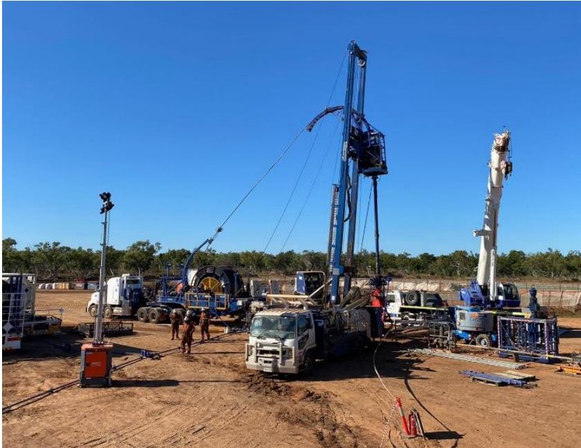
Coil Tubing Unit rigged up during well cleanout operations
