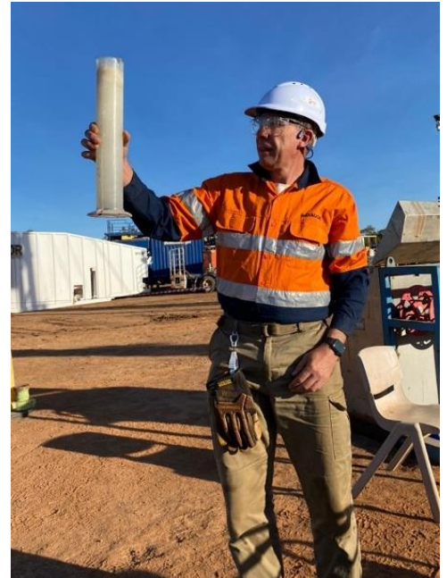
Senior Stimulation Engineer Daniel Kalinin inspecting gas bubbling in freshly sampled flowback fluid
