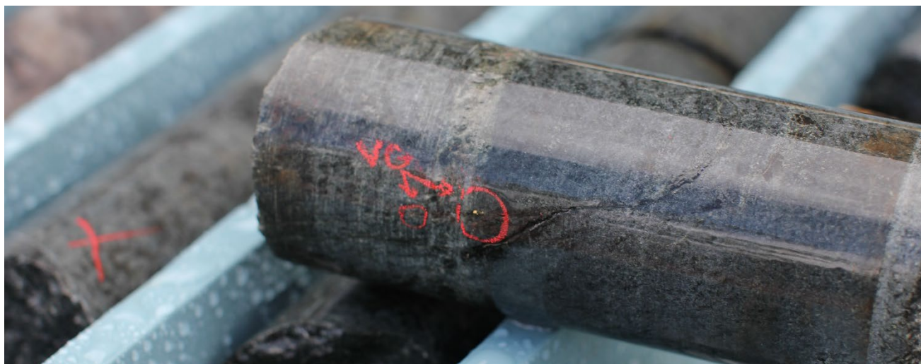
Figure 2 - Visible gold occurrence in RBDD005 drill-core (NQ), at 192.5m. Visible gold does not characterise all mineralised intercepts at Redback. The former owner reported visible gold was encountered in several drill-holes. These have been validated both by observation of remaining core and core photos.
