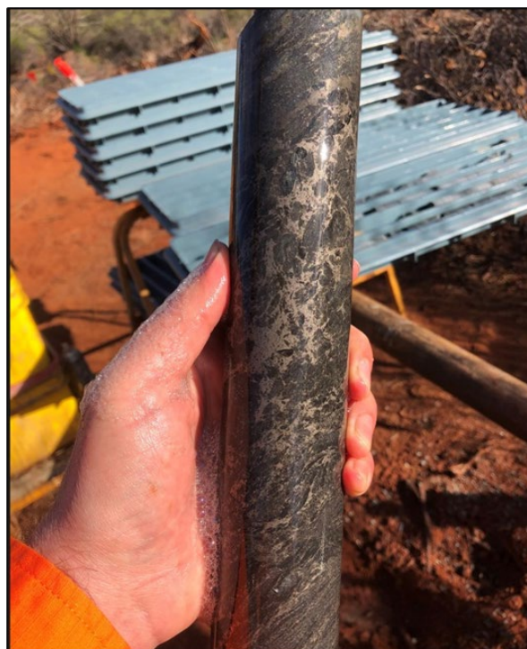
Figure 8 –Left- Wattle Dam East - Down Hole EM (DHEM) survey results. (Po – pyrrhotite). Right - Significant pyrrhotite mineralisation from 504.5m. NQ sized core.
