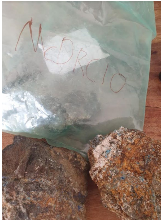
Figure 4: McDRC10 – Float sample of mineralized weathered granitic material derived from workings developed in a gully draining McDonalds area assaying 3.84% Copper and 4.25% Tin
