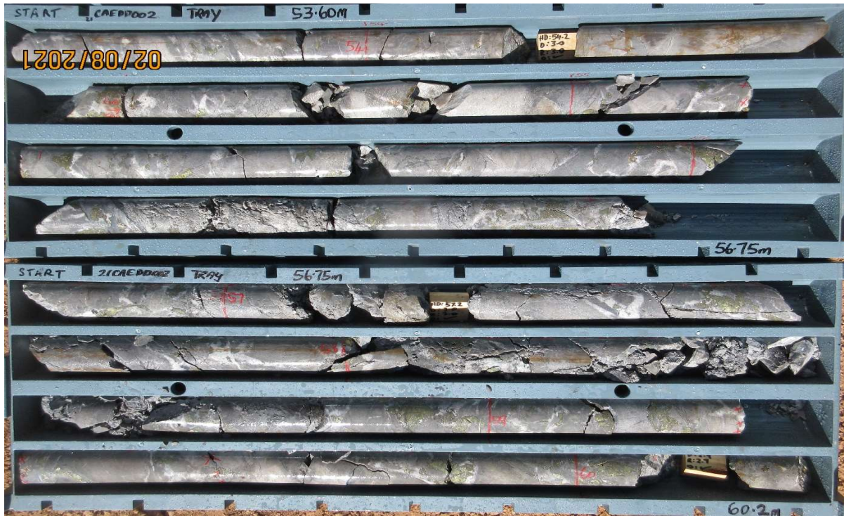
Figure 2. Continuation of hydrothermally breccia with chalcopyrite infill between hornfelsed sediment and felsic intrusive clasts.
