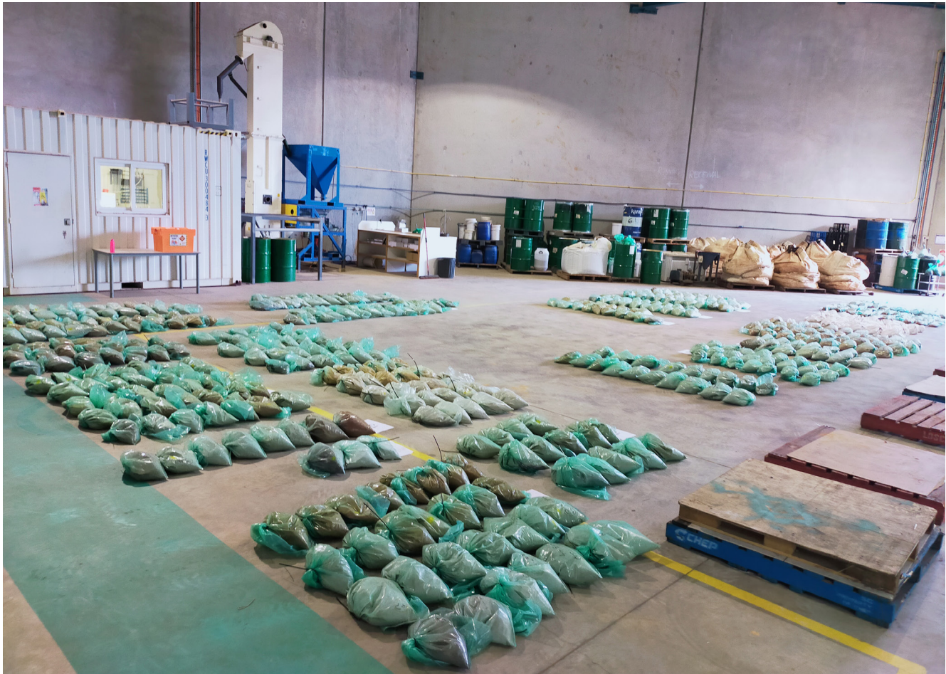
Figure 11: As-received drill samples
