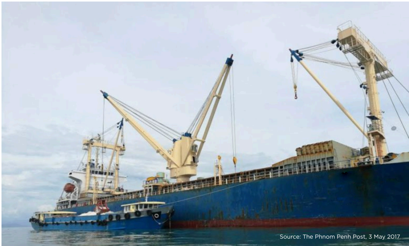
Figure 20: An example of silica sand being loaded from a barge to a bulk carrier using a grab crane
