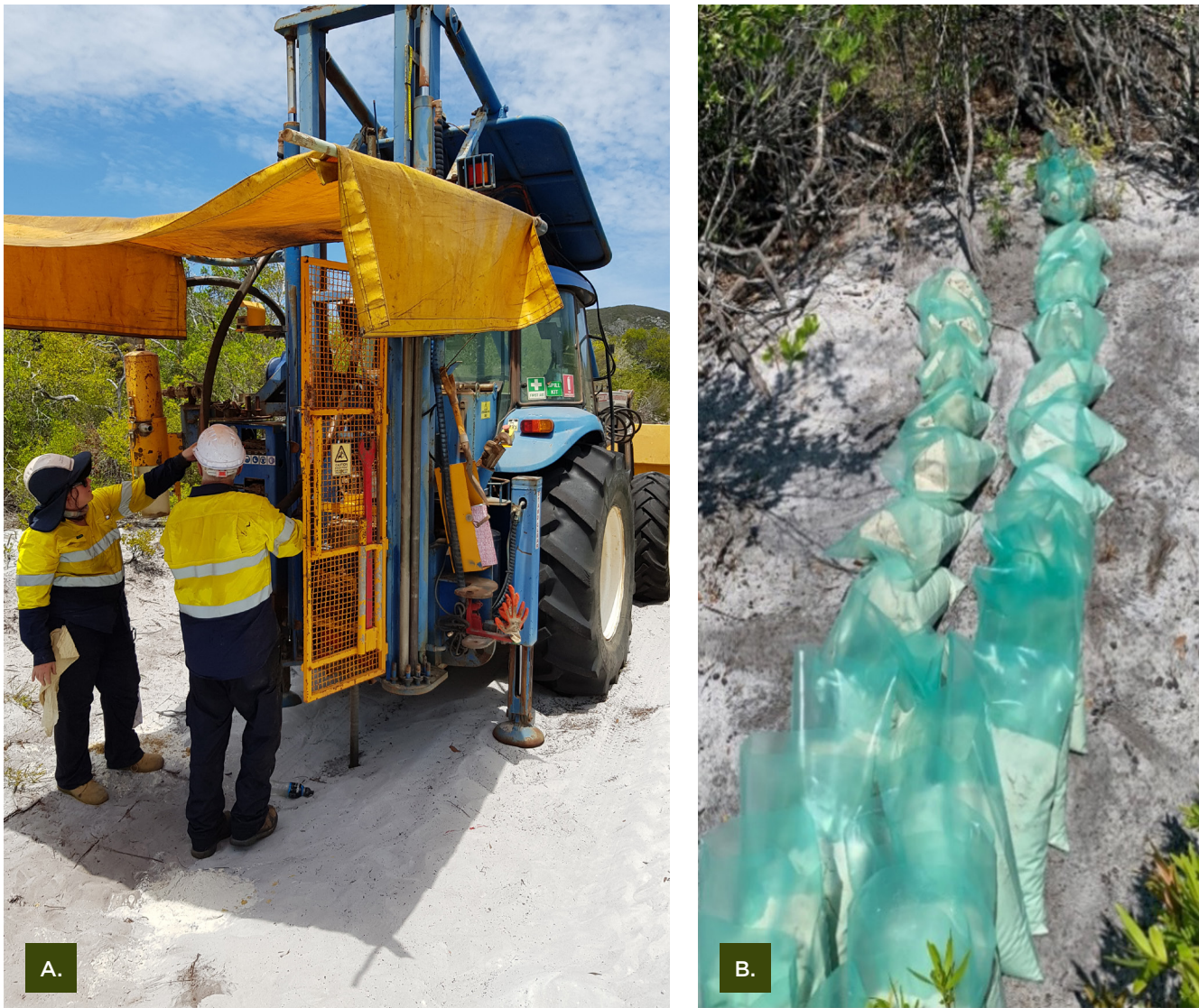
Figure 9: A. A vacuum drill rig in operation at site, and B. Collected and bagged sand samples
