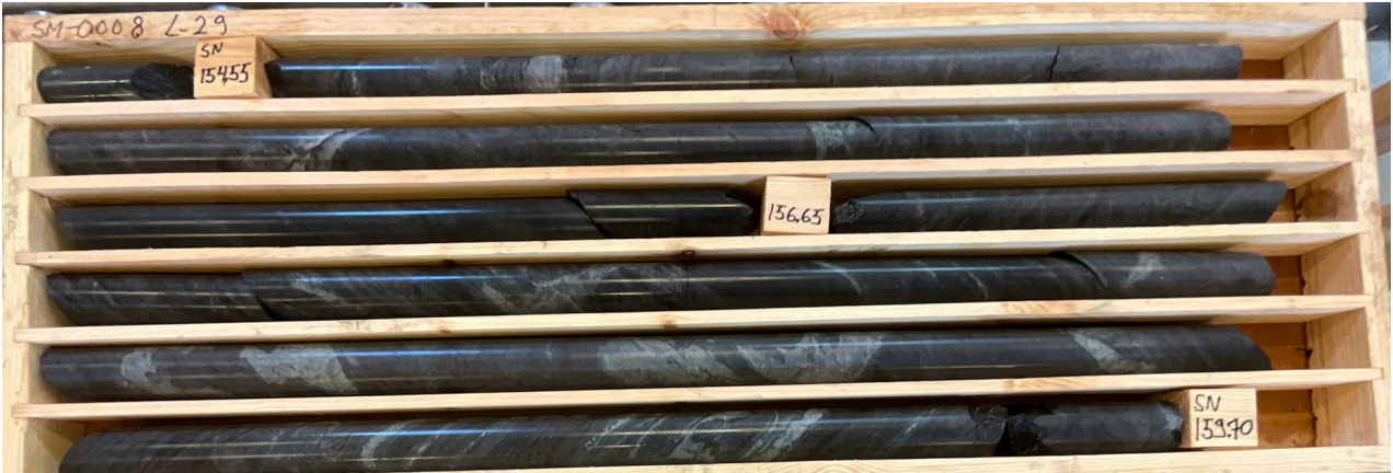
Figure 3: Diamond drillhole SM0008 (154.45m – 159.70m) at Satulinmäki. Multiple calc-silicate veins and alteration halos with associated weak to moderate pyrrhotite mineralisation and trace arsenopyrite. Indicators of potential Gold mineralisation.
