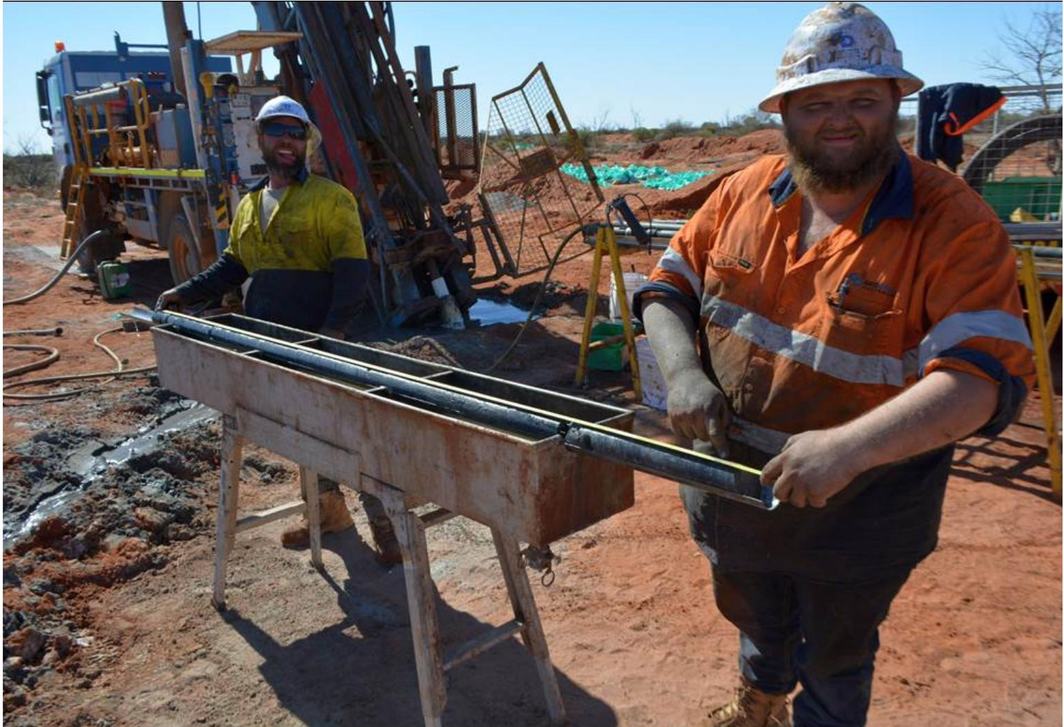
**Figure 2:** Marmota extends its thanks to the members of the drill crew rig (here with a 2.7m length of core featuring 100% recovery)
