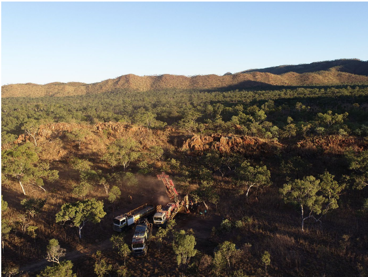
Figure 8: RC drilling KMRC016 at the Grant’s Find target showing the outcropping copper-gold lode. Orion in the middle-ground and Rough Triangle in the background.
