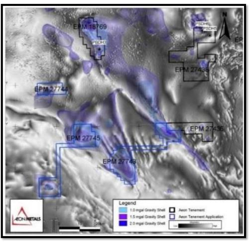
Aeon tenements with 3D inverted gravity shells and BW magnetics underlain
