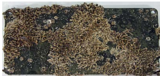
Ablative marine coating – no additive
