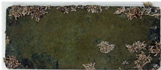
Ablative marine coating – 200 g /L Calix additive
