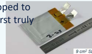
Single layered pouch (SLP) cell prepared by Qinetiq featuring Calix LMO cathode
