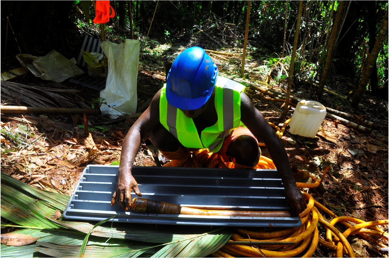
Figure 4 – Local Driller loading core from Stage 2 Drilling
