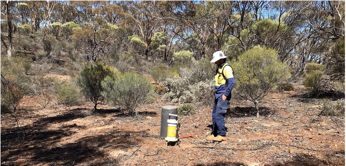
Figure 3 - GAP Geophysics crew onsite at the Central Prospect, showing SQUID equipment in action.
