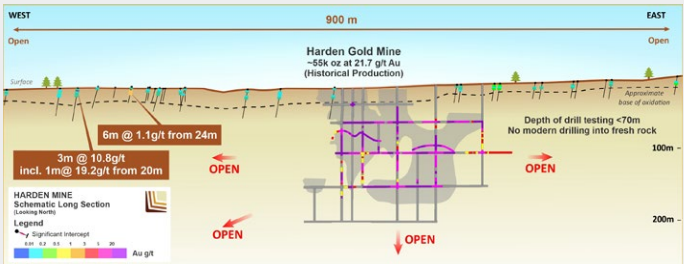
Figure 13: Harden Mine long-section showing historical drilling, production and working
