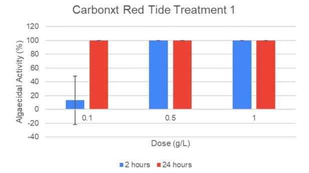
Figure 2: Alternative algaecide/activated carbon composite results
