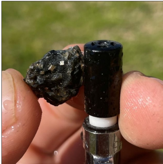
Figure 2: RC chip from drillhole RC21HN003 66-67m containing disseminated pyrite
