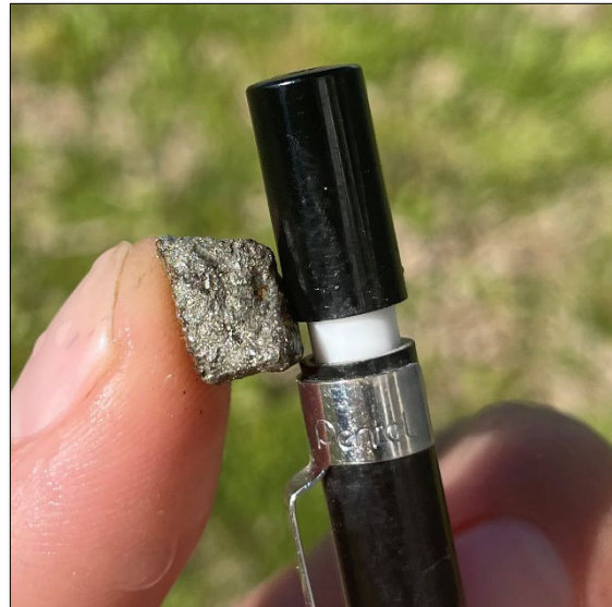
Figure 3: RC chip from drillhole RC21HN007 63-64m containing disseminated and veined pyrite
