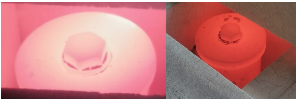
Figure 1. Retort casing at end of test run showing “white hot” cannister.
