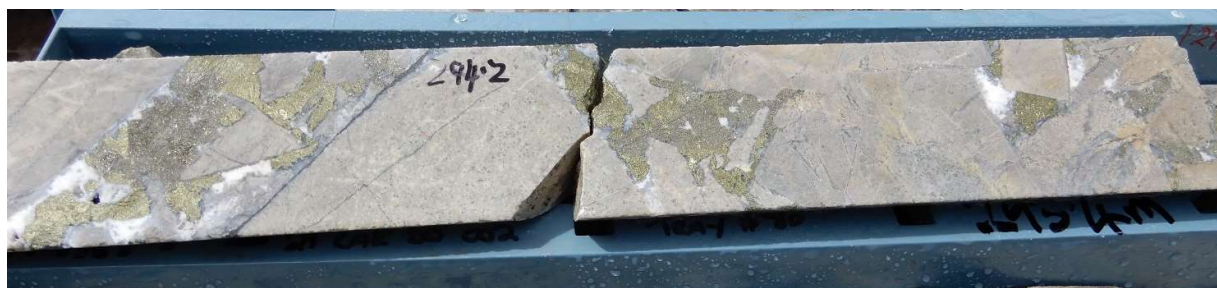
Fig 15. Primary copper mineralisation Hole 21CAEDD002, 294.2m , -8% visual estimate of chalcopyrite in the interval 294m-295m, Assay results awaited.
