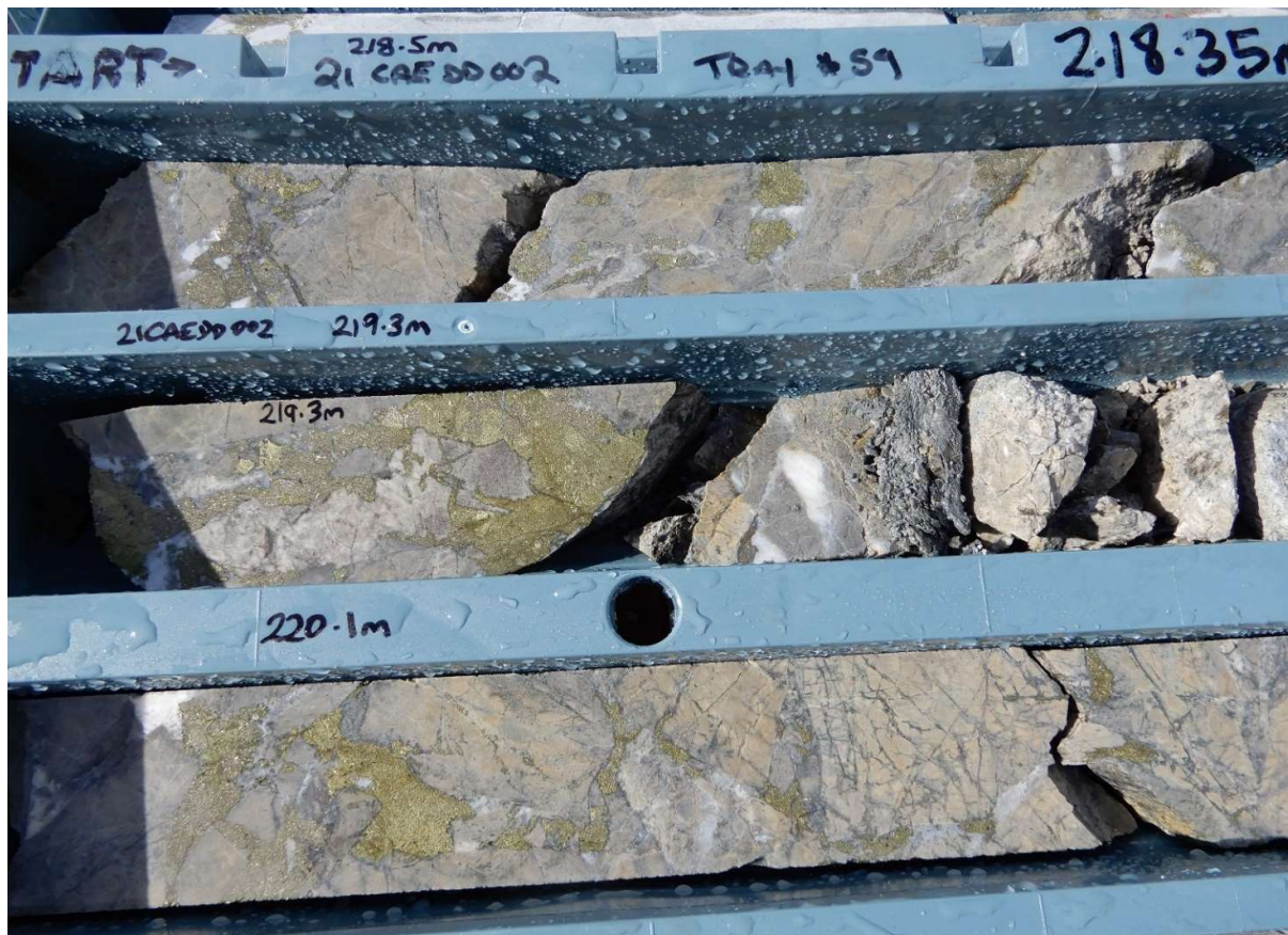
Fig 12. Primary copper mineralisation Hole 21CAEDD002 , 219,220m ,8%-10% visual estimate of chalcopyrite in the interval 219m-221m. Assay results awaited.
