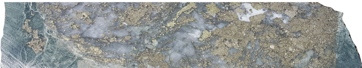
Figure 3. High grade drill intersection of quartz-carbonate-pyrite-chalcopyrite in DTDD004 (215.4 – 215.9m) that reported 0.5m @ 9.57 g/t Au, 16.8 g/t Ag and 0.68% Cu.
