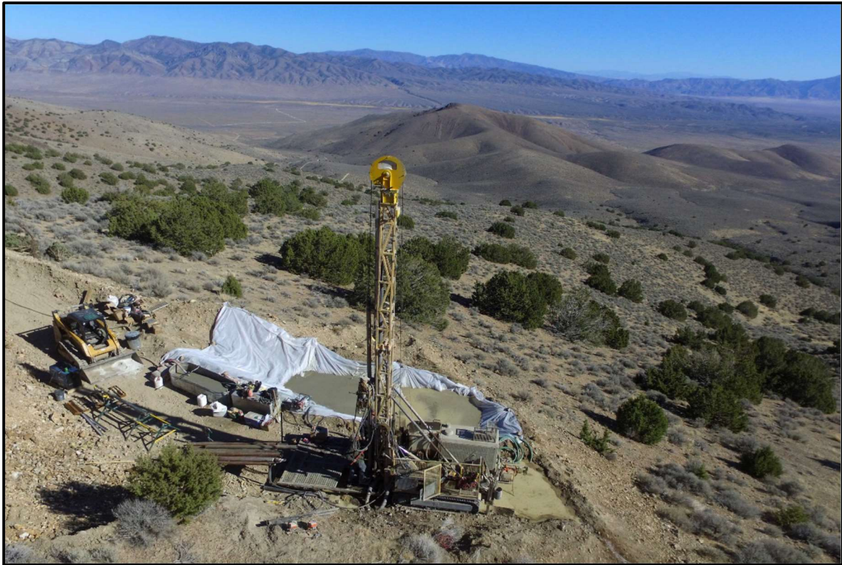
Figure 7: Diamond Drilling Rig on site at Lambarson Canyon project, Nevada
