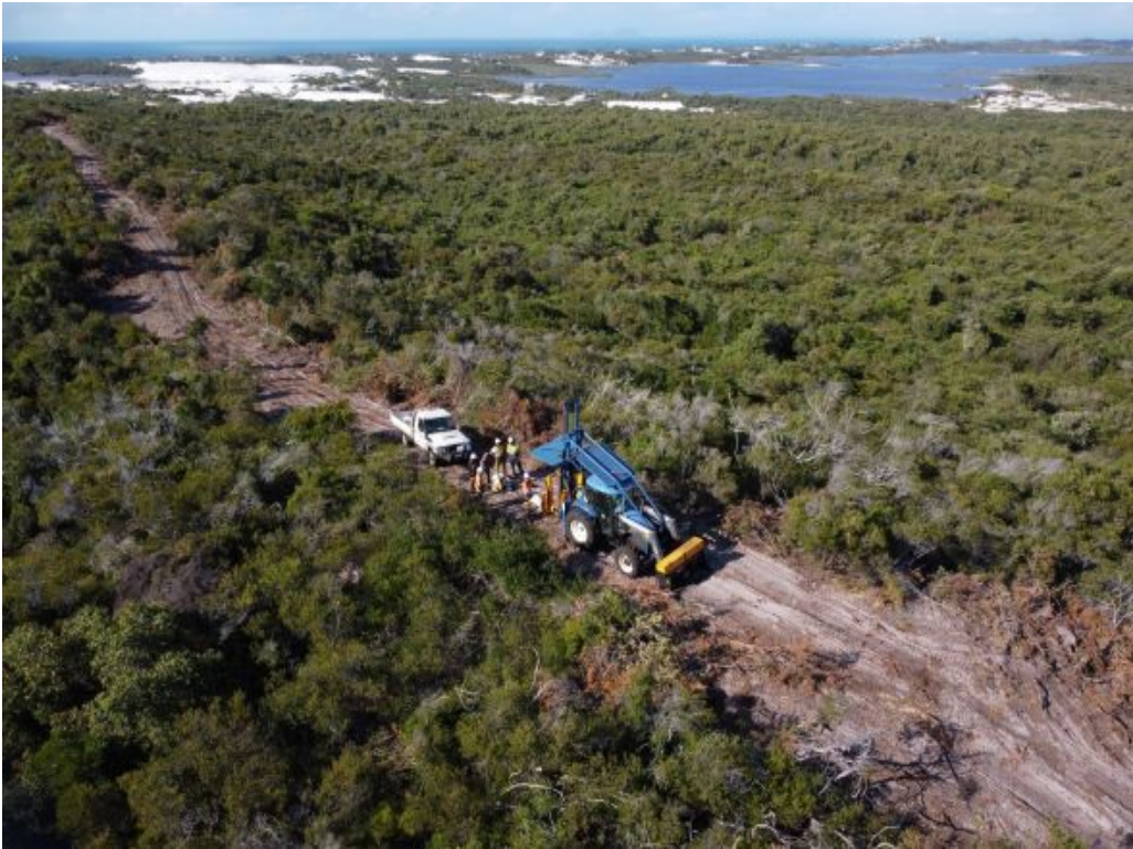
Figure 4. Yearlong Contractors vacuum-based drill rig working at CFS project with Mitsubishi silica sand operations in the background
