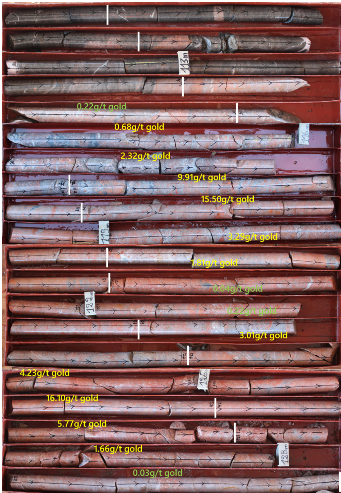
Figure 14: DSDD020 (111-128.96m) core showing mineralised zone on the SWF2 structure. Alteration and hydrothermal brecciation commences from 112.90m with strongly defined qtz-carb-pyr-tourmaline matrix in upper section. Strong albite-hem-Fe carb-qtz alteration throughout mineralised zone, with minor coarse pyrite agglomerations typically present in the high-grade NW-SE dilational fault.
