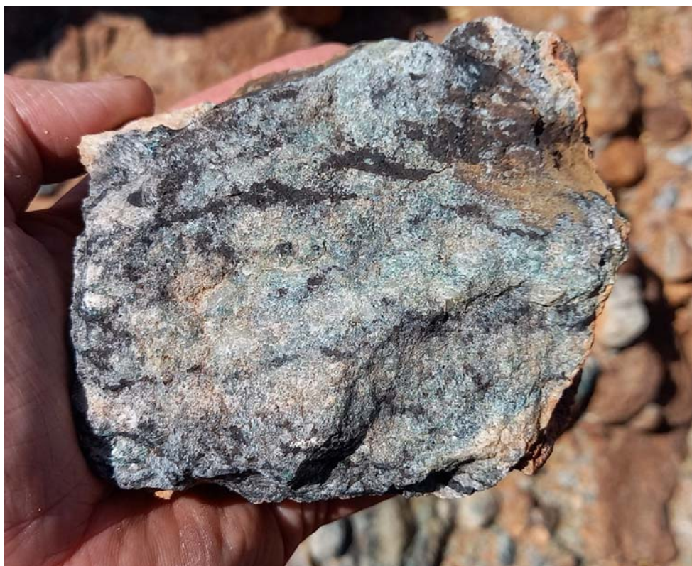
Figure 4. Chalcocite & malachite bearing barite. (Sample # ZEU021).
