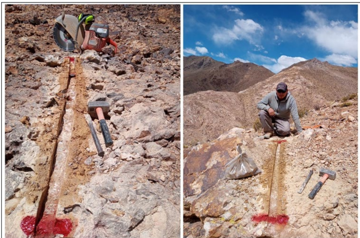
Figure 3 – Example of the channel sampling undertaken across the northern geophysical anomaly at the at Las Opeñas Gold Project
