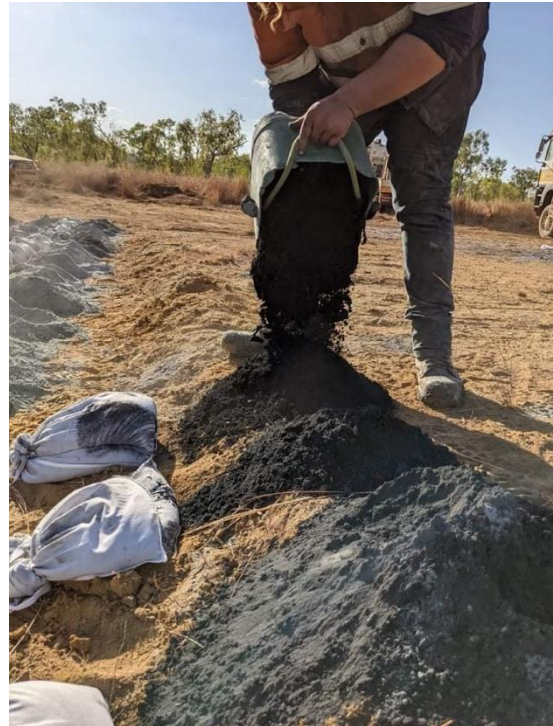
Figure 8: 1m RC piles of massive sulphide mineralisation from KMRC026.
