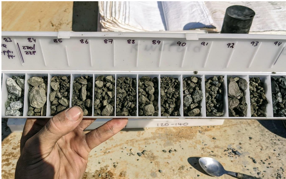
Figure 5: Chip tray from KMRC019 showing the 12m of pyrite-dominant massive sulphide from 83m, which contained 2 – 10% chalcopyrite.
