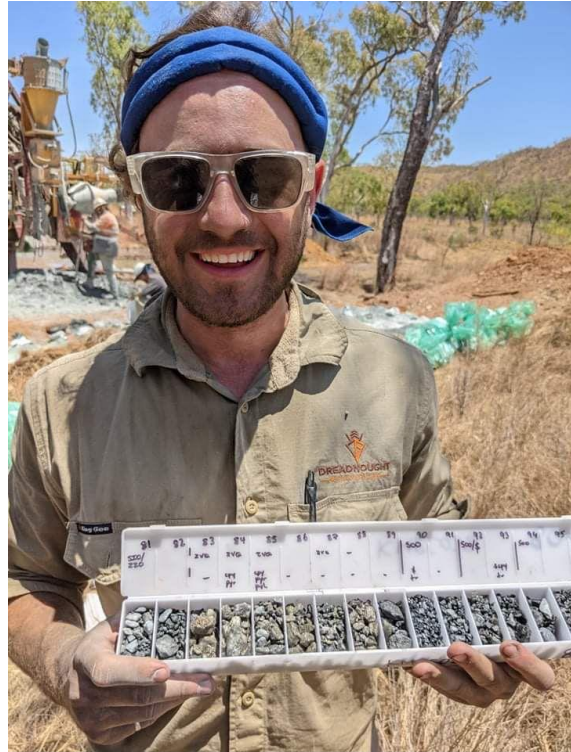
Figure 6: Dreadnought's Luke Blais holding a chip tray from KMRC022 showing the highly enriched 5m of 15-25% chalcopyrite from 82m.
