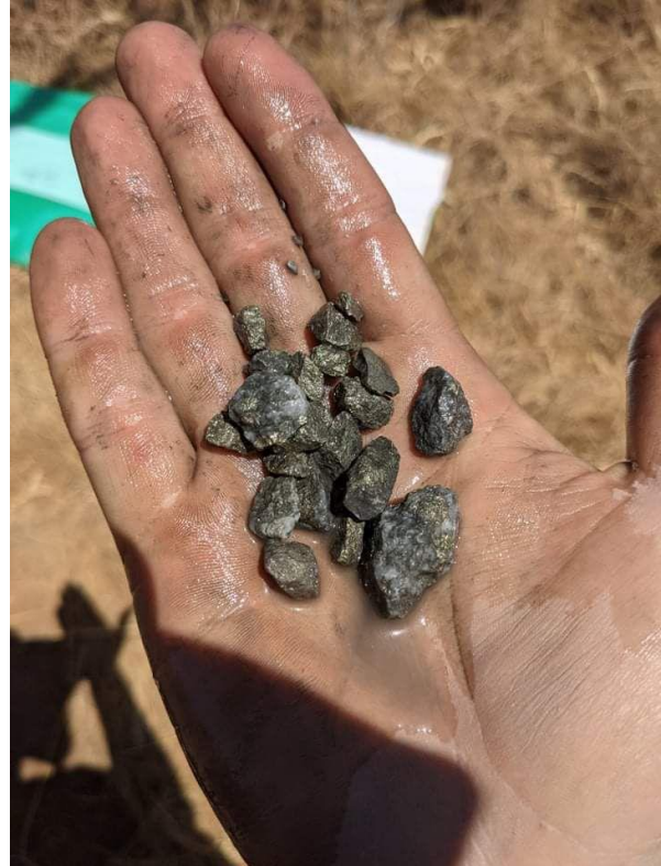
Figure 4: Semi-massive sulphide quartz breccia chips from KMRC019 drilled down dip of KMRC017 showing Cu-Ag bearing massive sulphides from 83m.
