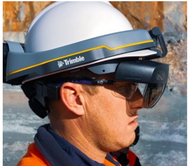
HoloLens (Augmented Reality) technology at Cowal - enables maintenance teams on the surface and/or at the Original Equipment Manufacturer or Dealership to view what the maintainer is seeing in real-time to expedite troubleshooting eg working on an excavator in the open pit
