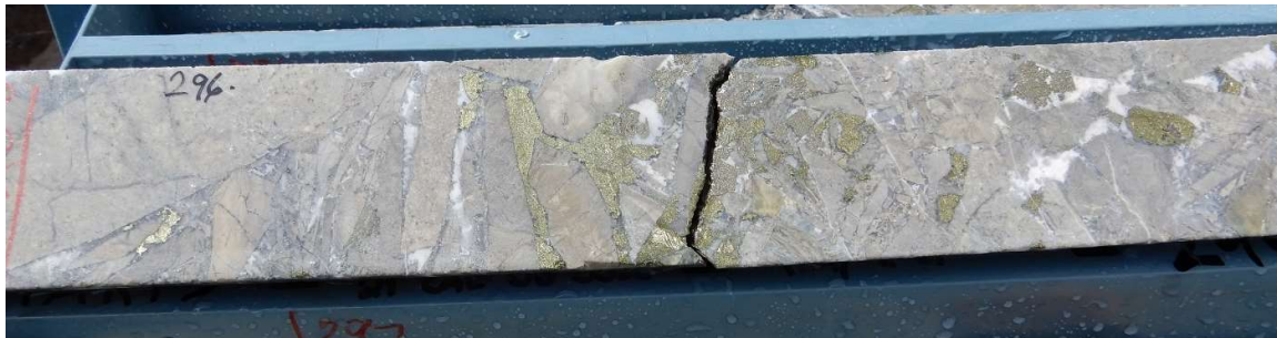
Fig 12. Primary copper mineralisation Hole 21CAEDD002 , 296m , -8% visual estimate of chalcopyrite in the interval 296m-297m,, Lab assay result 1.50% Cu.
