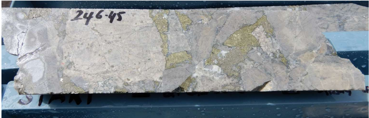
Fig 9. Primary copper mineralisation Hole 21CAEDD002 , 246.45m , -3% visual estimate of chalcopyrite in the interval 246m-247m, Lab assay result 1.65% Cu.
