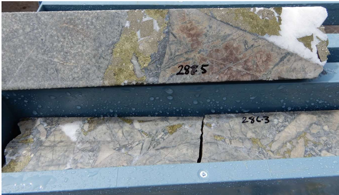
Fig 10. Primary copper mineralisation Hole 21CAEDD002, 288.5m , -5% visual estimate of chalcopyrite in the interval 288m-289m, Lab assay result 2.10% Cu.
