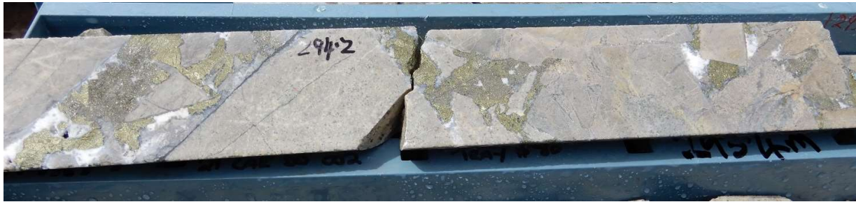
Fig 11. Primary copper mineralisation Hole 21CAEDD002, 294.2m, -8% visual estimate of chalcopyrite in the interval 294m-295m, Lab assay result 2.00% Cu
