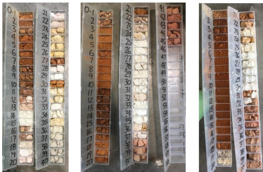
Plate 1: Photos of rock chip trays showing rock chip samples from one metre intervals in drill holes FRAC 19-04 (left), FRAC 19-16 (middle) and FRAC 19-21 (right).
