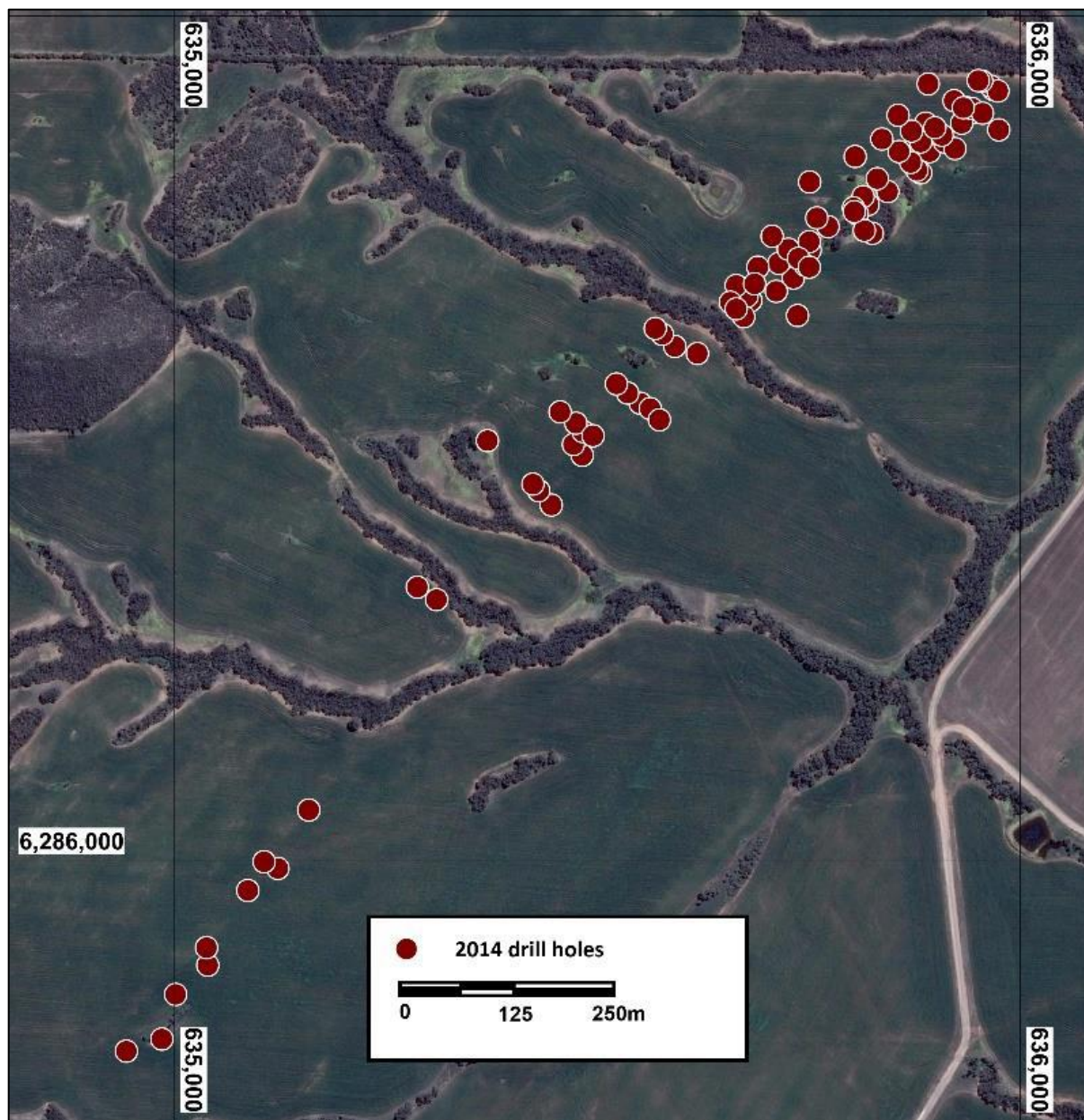
Figure 5. Plan showing location of Central Campoona resource drill holes.
