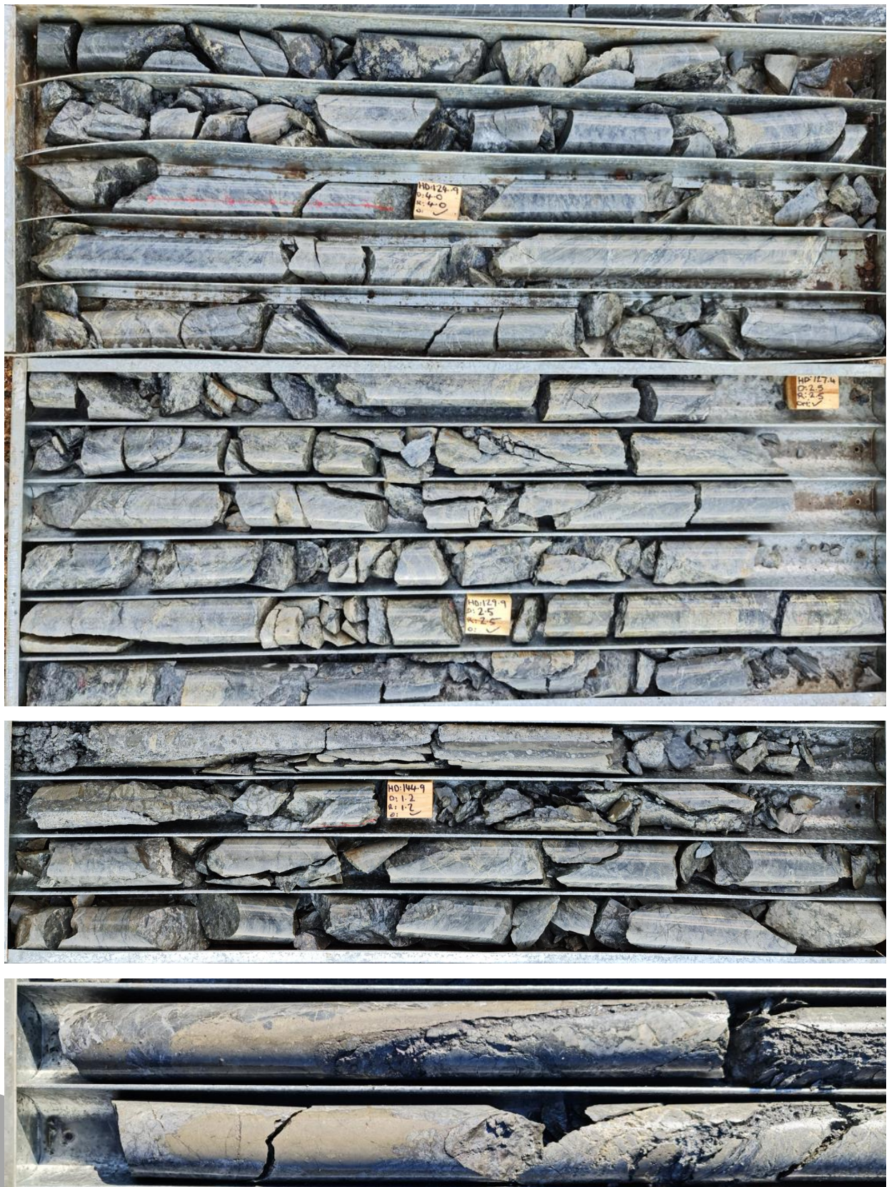
Figure 6 – Examples of veined and brecciated phyllic altered sandstone with 5-10% mixed sulphides throughout (from 126m-187m RDD003). Hole is continuing to at least 400m.
