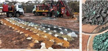
Drill rig at HWRC003 (left) with sieved chips showing contrast between mineralised structure and fuchsite alteration halo (right)
