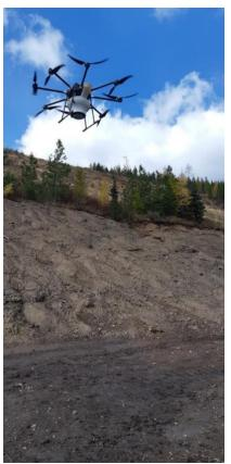
Figure 3: Drone at application altitude delivering to Fernie mined area
