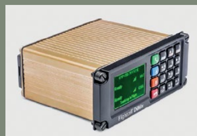
Flightcell DZMx – satellite communications and tracking device
