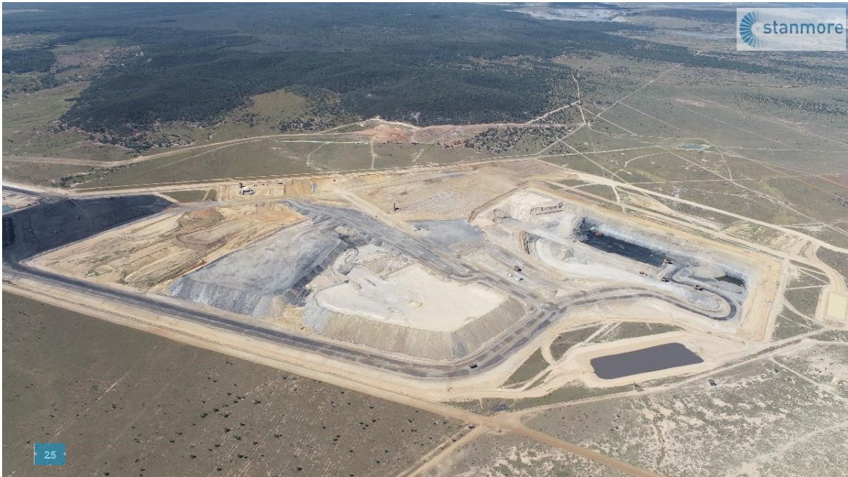
Figure 1: Isaac Downs bulk sample pit, ROM stockpile on the left, and Millennium mine in the far background
