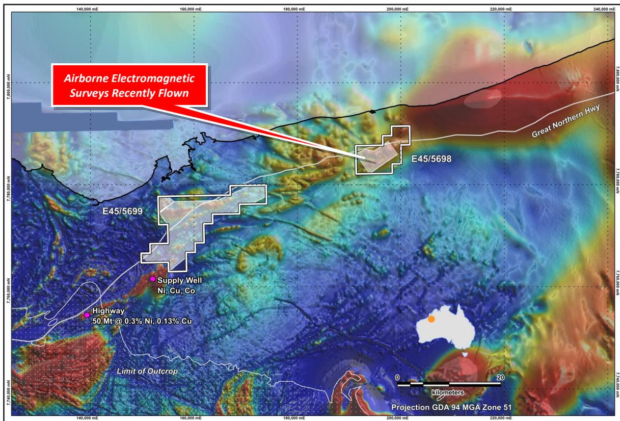
[Figure 8] Pardoo Nickel Project: Regional magnetic image with Red Metal tenement locations and the known Highway and Supply Well nickel prospects (pink circles). The frosted region identifies the planned airborne electromagnetic survey area due to start in about one month, following completion of the current Yarrie survey.
