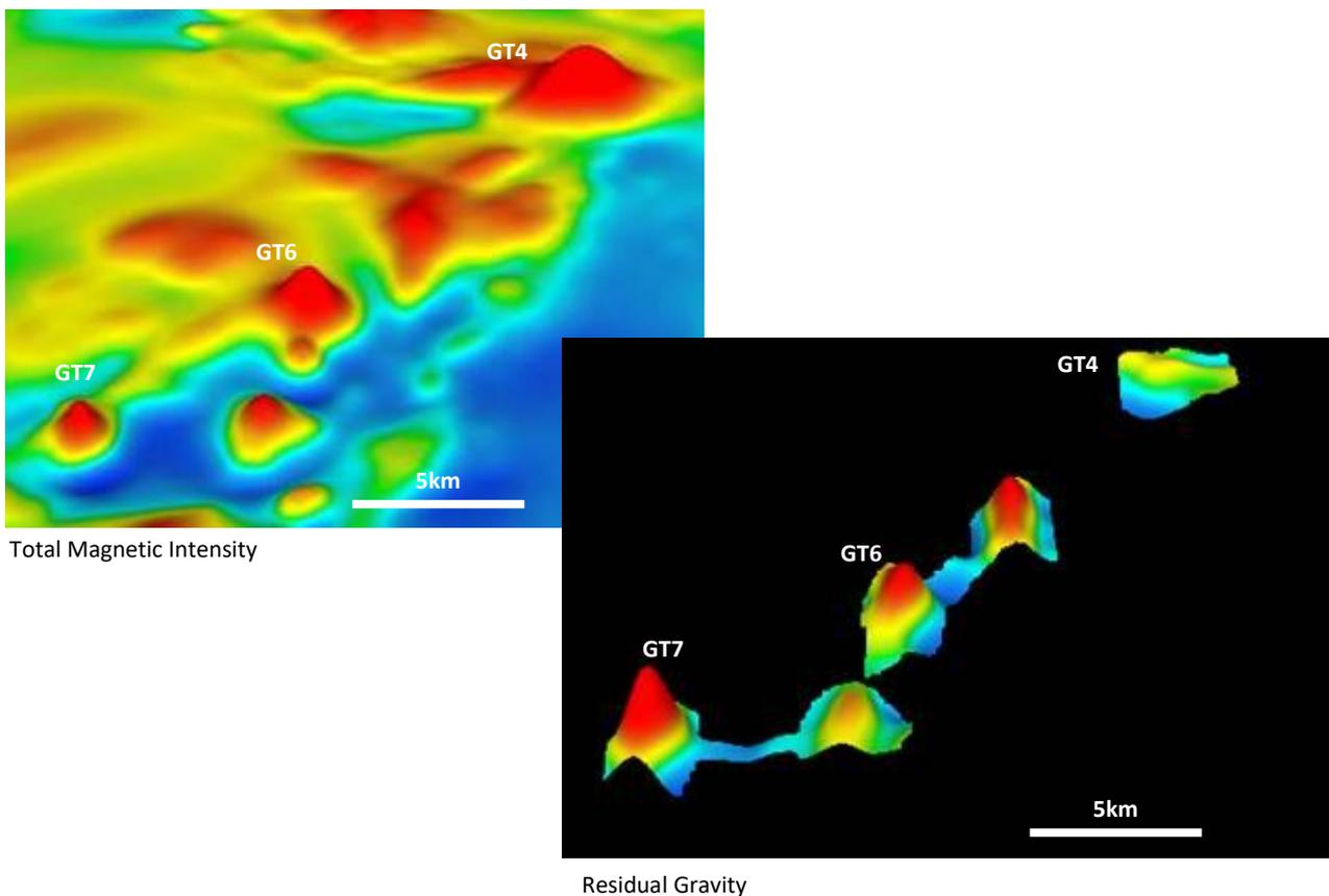
[Figure 3] Gulf Project: Gibson's Tank 3D oblique topographic view of the total magnetic intensity (top left) and the residual gravity from Red Metal's surveying (bottom right). Key targets for drill testing in 2021 include the high magnetic and high gravity targets GT7 and the high magnetic, weak gravity target GT4.
