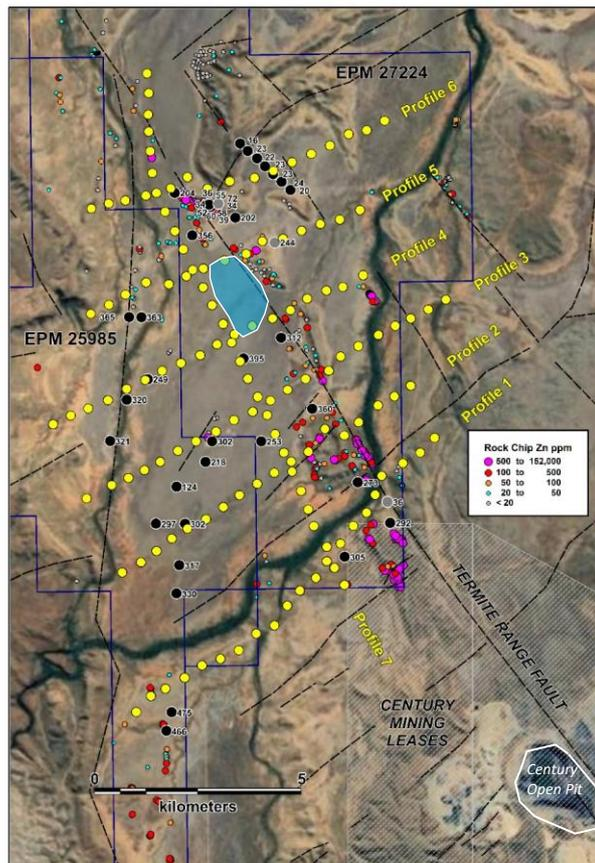
[Figure 6] Lawn Hill Project, Century North tenements: Satellite image showing magnetotelluric stations (yellow dots), historic drilling with end of hole depth labelled (black) and thematic zinc in surface rock chips. Prospective area offering potential for preservation of Century age stratigraphy adjacent to the Termite Range Fault is shown as a blue polygon.
