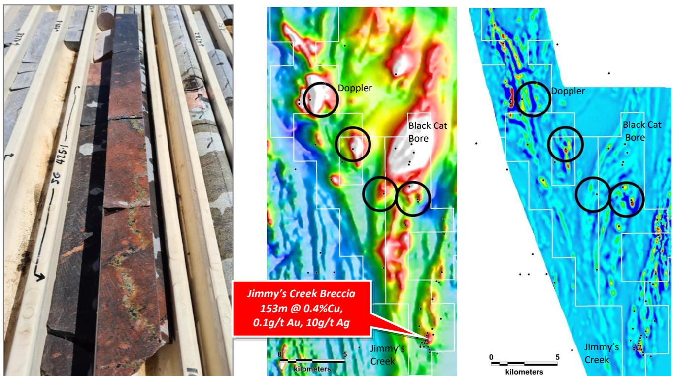
[Figure 10] Corkwood Project: Porphyritic volcanic rock showing early magnetite-biotite alteration (black colour at the top) demagnetised by red feldspar-silica alteration and associated chalcopyrite (weak magnetite) veining (left). Total magnetic intensity image highlighting high magnetic alteration zones (centre). The vertical gradient magnetic imagery highlights low magnetic regions within or adjacent to the high magnetic alteration zones which will be targeted for copper-gold mineralisation.
