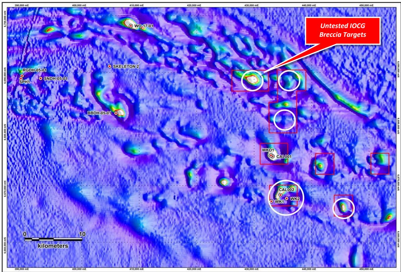
[Figure 13] Callabonna Joint Venture Project: Magnetic intensity image showing existing drill holes and the main untested magnetic and gravity targets proposed for further evaluation and drilling (white circles).
