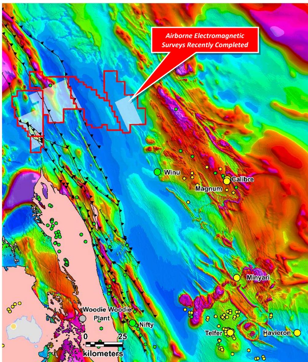
[Figure 1] Paterson Province Yarrie Project: Magnetic imagery overlain by the recently flown airborne electromagnetic survey area (frosted white) showing the Nifty mine, Telfer mine, new Winu and Haverion discoveries and Red Metal's Yarrie tenements (red line). Note the exposed basement terrain of older Archaean rocks (buff coloured polygon).
