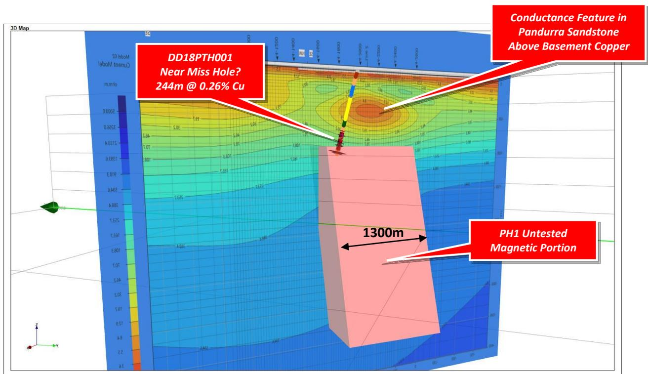
[Figure 11] Punt Hill and Pernatty Lagoon Project: PH1 target, 3D oblique view facing northwest showing the preliminary conductance depth inversion image and the 3D magnetic model and near miss drill hole DD18PTH001. Note the significant dimension of the modelled magnetic target and the high conductance feature in the cover sequence directly above the untested portion of the model.
