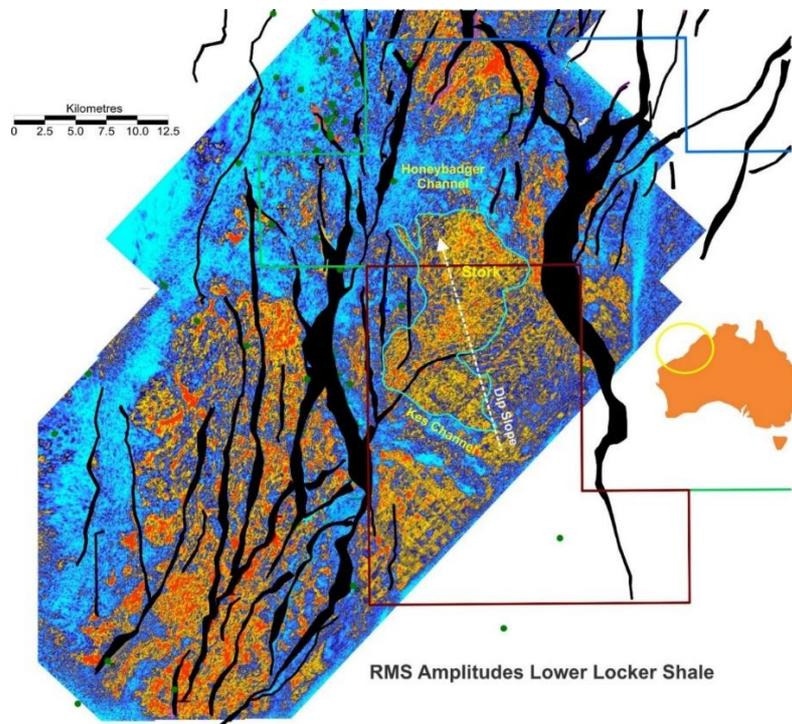
Higher seismic amplitudes (warm colours) define the deltaic sands in the Lower part of the Locker Shale which form the reservoir at Dorado; the clay seals (cold colours) by the Kes Canyon and the erosion of the sand package by the Honeybadger canyon clearly define the prospect.
