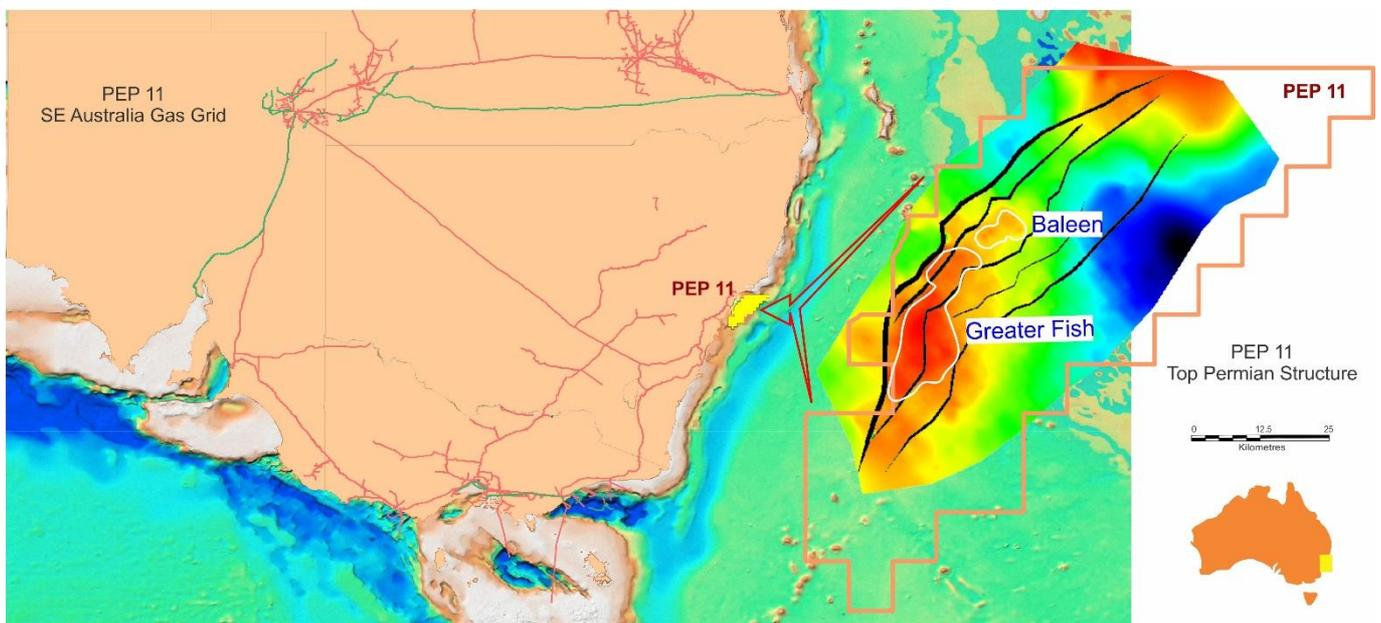
A 200km 2D seismic survey was completed in March 2018 in the area of the Baleen prospect and with AVO analysis further refined the Baleen target located 30 km southeast of Newcastle.
