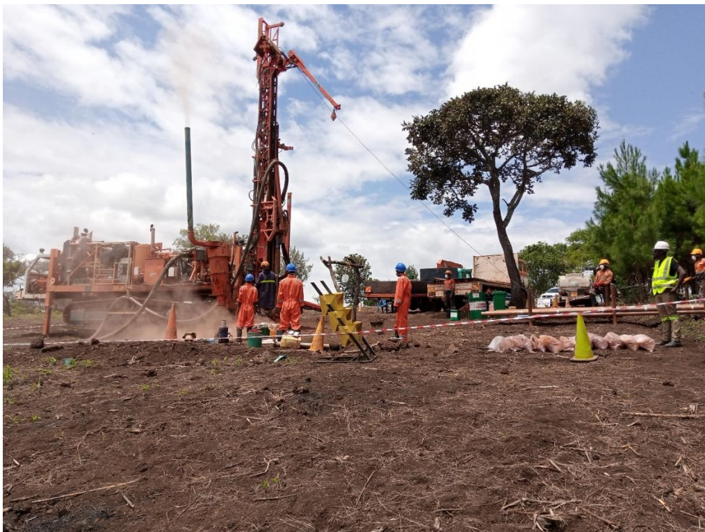
Image 2 – RC drilling operations underway at Target 20
