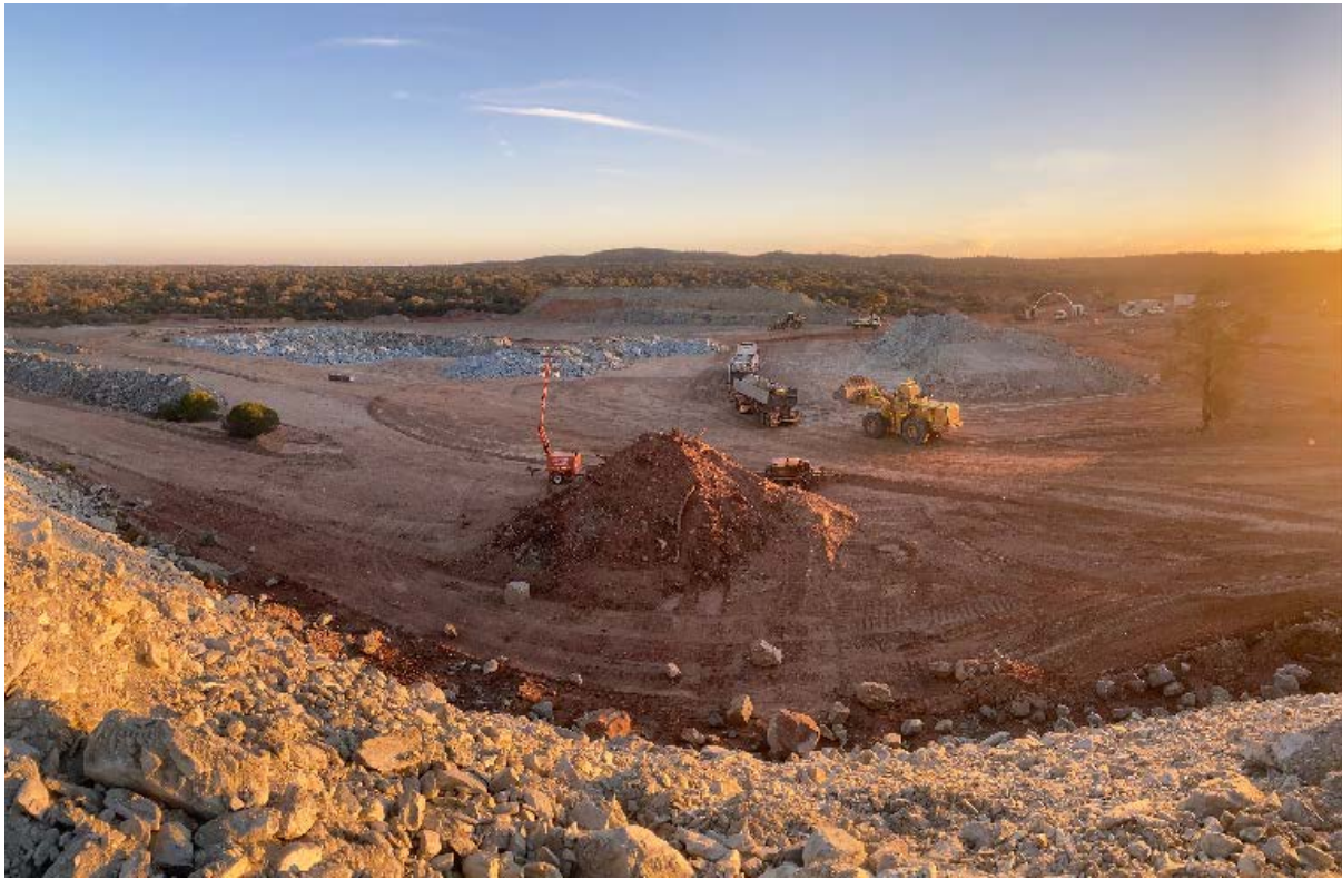
Plate 2 Panorama showing ROM stockpiles High Grade (right) and Low-grade (Left) ore fingers
