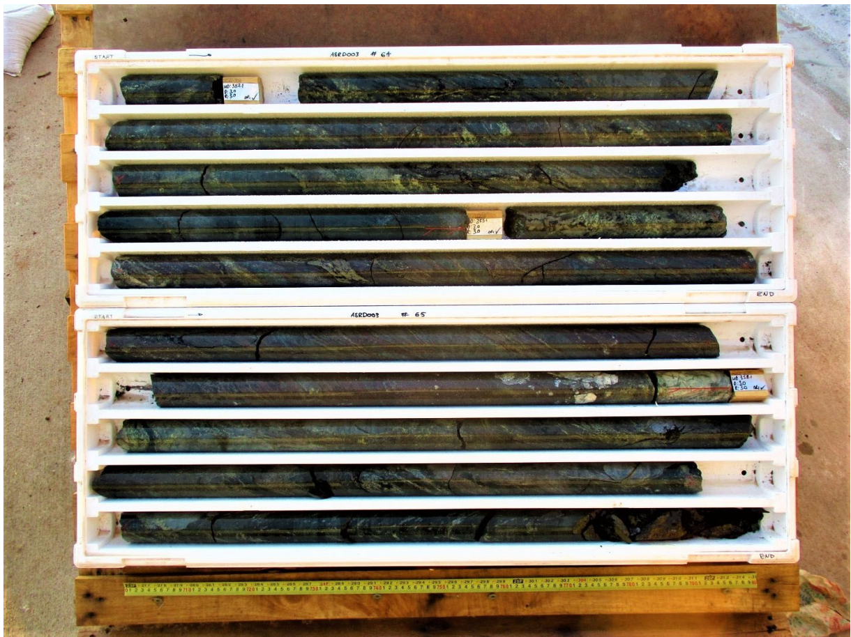
Figure 6 – Diamond core samples from ASRD003 at 355m
