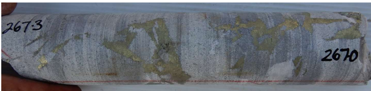
Fig 11. Primary copper mineralisation Hole 21CAEDD003 , 267m-268m , 10% visual estimate of chalcopyrite in the interval 63m-64m. Lab assay result 2.72% Cu, 0.36 g/t Au, 54 g/t Ag.
