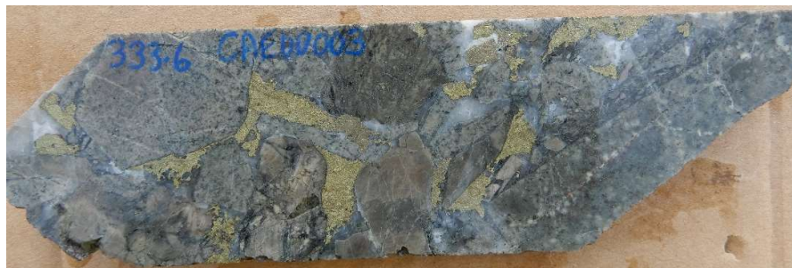
Fig 12. Primary copper mineralisation Hole 21CAEDD003 333.6m , 8% visual estimate of chalcopyrite in the interval 333m-334m. Lab assay result 2.29 % Cu, 0.96 g/t Au, 54 g/t Ag. Hosted in infill polymict breccia, clasts hornfels,diorite, infill matrix carbonate , quartz, pyrite.
