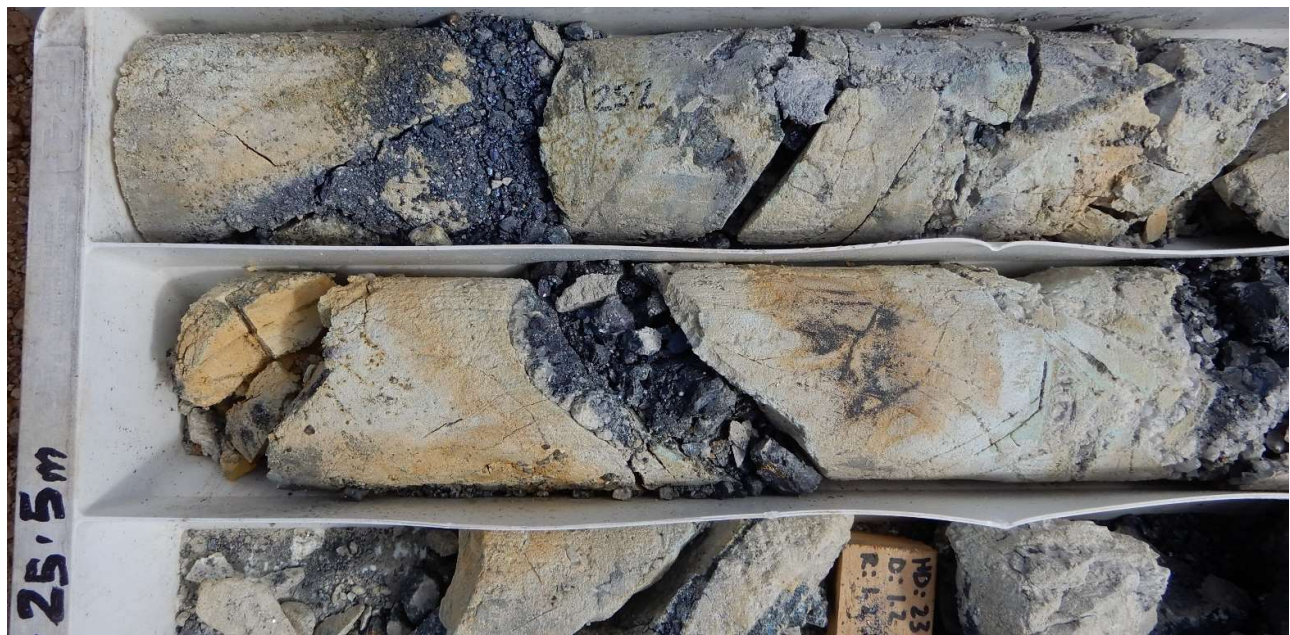
Fig 9. Supergene copper mineralisation Hole 21CAEDD003 ,15% visual estimate of chalcocite in the intervals 24m-25m, Lab assay result 24m-24.5m 8.86% Cu, 64 g/t Ag,2.52 g/t Au. 24.5m-25.0m 5.93% Cu, 52 g/t Ag,2.60 g/t Au.
