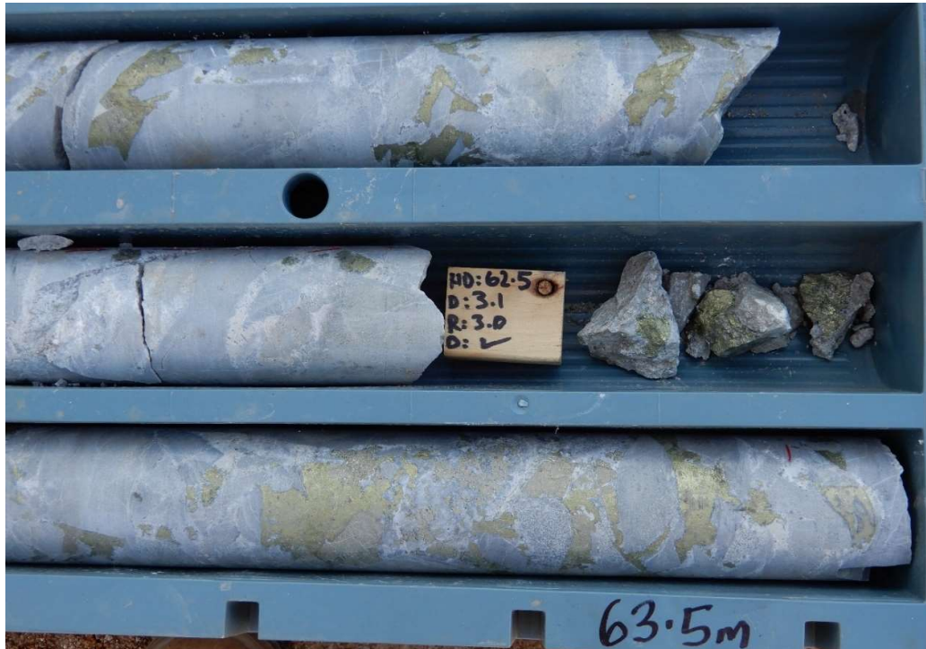
Fig 10. Primary copper mineralisation Hole 21CAEDD003 , 62m-64m , 10% visual estimate of chalcopyrite in the interval 63m-64m. Lab assay result 4.47% Cu, 0.86 g/t Au, 64 g/t Ag
