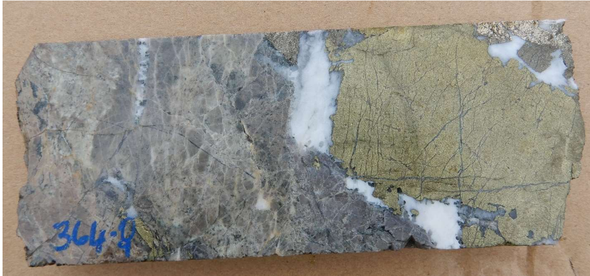
Fig 13. Primary copper mineralisation Hole 21CAEDD003 364.9m , 10% visual estimate of chalcopyrite in the interval 334m-365m. Lab assay result 6.05 % Cu, 0.64 g/t Au, 62 g/t Ag. Hosted in infill breccia, clasts hornfels, infill matrix carbonate , quartz, pyrite.
