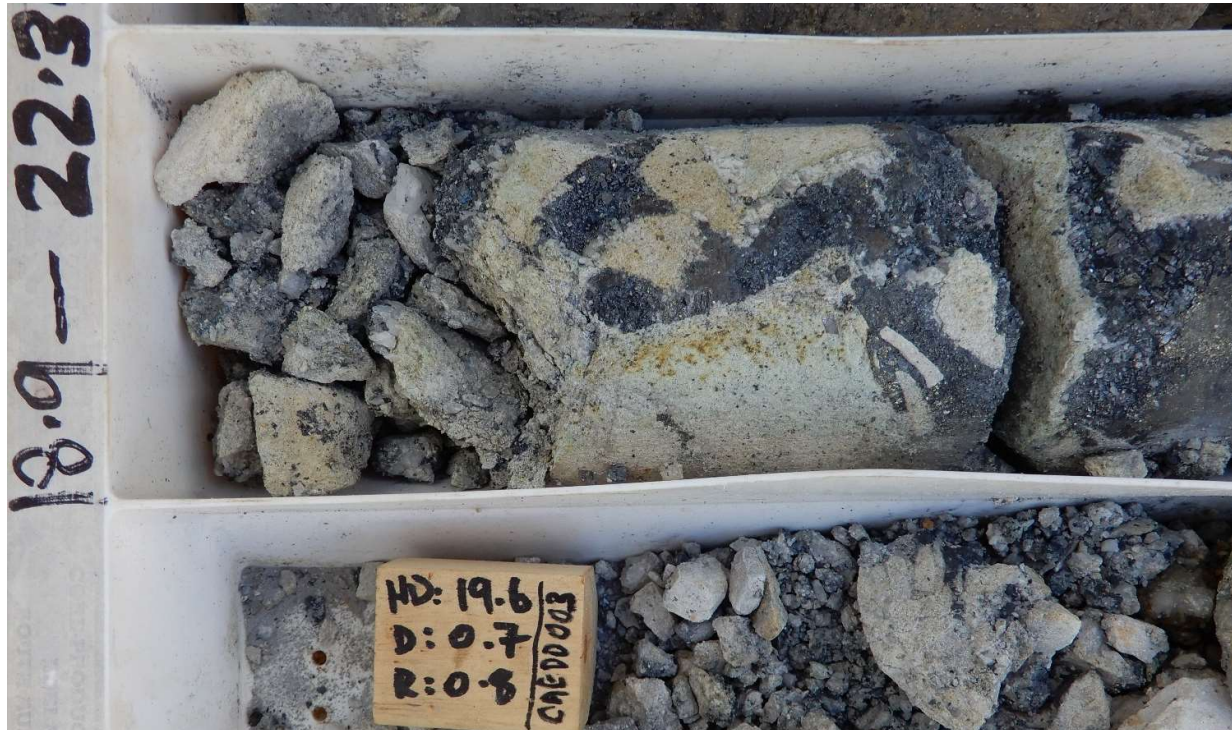
Fig 8. Supergene copper mineralisation Hole 21CAEDD003 ,10%-15% visual estimate of chalcocite in the intervals 19m-20m, Lab assay result 19m-19.5m 5.65% Cu, 59 g/t Ag,0.59 g/t Au. 19.5m-20.0m : 6.11% Cu, 34 g/t Ag,0.90 g/t Au.
