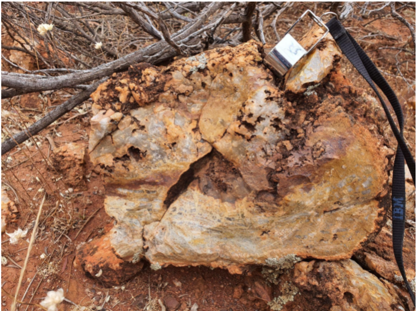
Figure 4: Example of outcropping hydrothermal quartz sulphide breccia with well developed boxwork
