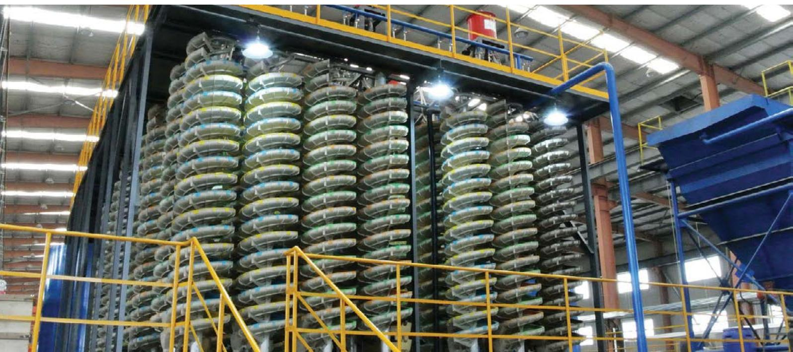
Spiral banks at Astron's Yingkou mineral separation plant, China.
