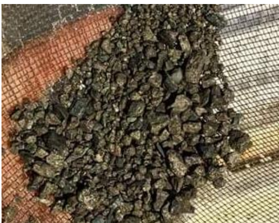
Figure 6: RC chips from KMRC022 84-85m showing massive sulphide mineralisation comprised of pyrrhotite-pyrite (bronze-yellow) and chalcopyrite (golden-yellow). This metre assayed 7.4% Cu, 132g/t Ag, 6.2 g/t Au.
