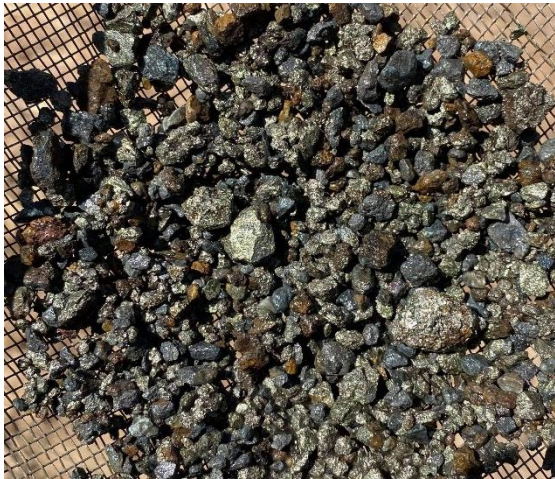
Figure 5: RC chips from KMRC039 18-19m showing supergene mineralisation comprised of chalcocite (dark grey) mixed with pyrite, chalcopyrite and gossanous iron oxides.
