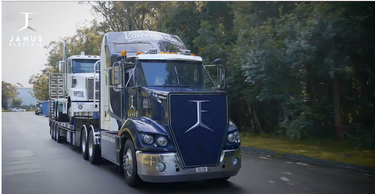
This Prime Mover was converted by Janus Electric and is operating with a Janus Electric Motor and exchangeable 600KWh battery pack
