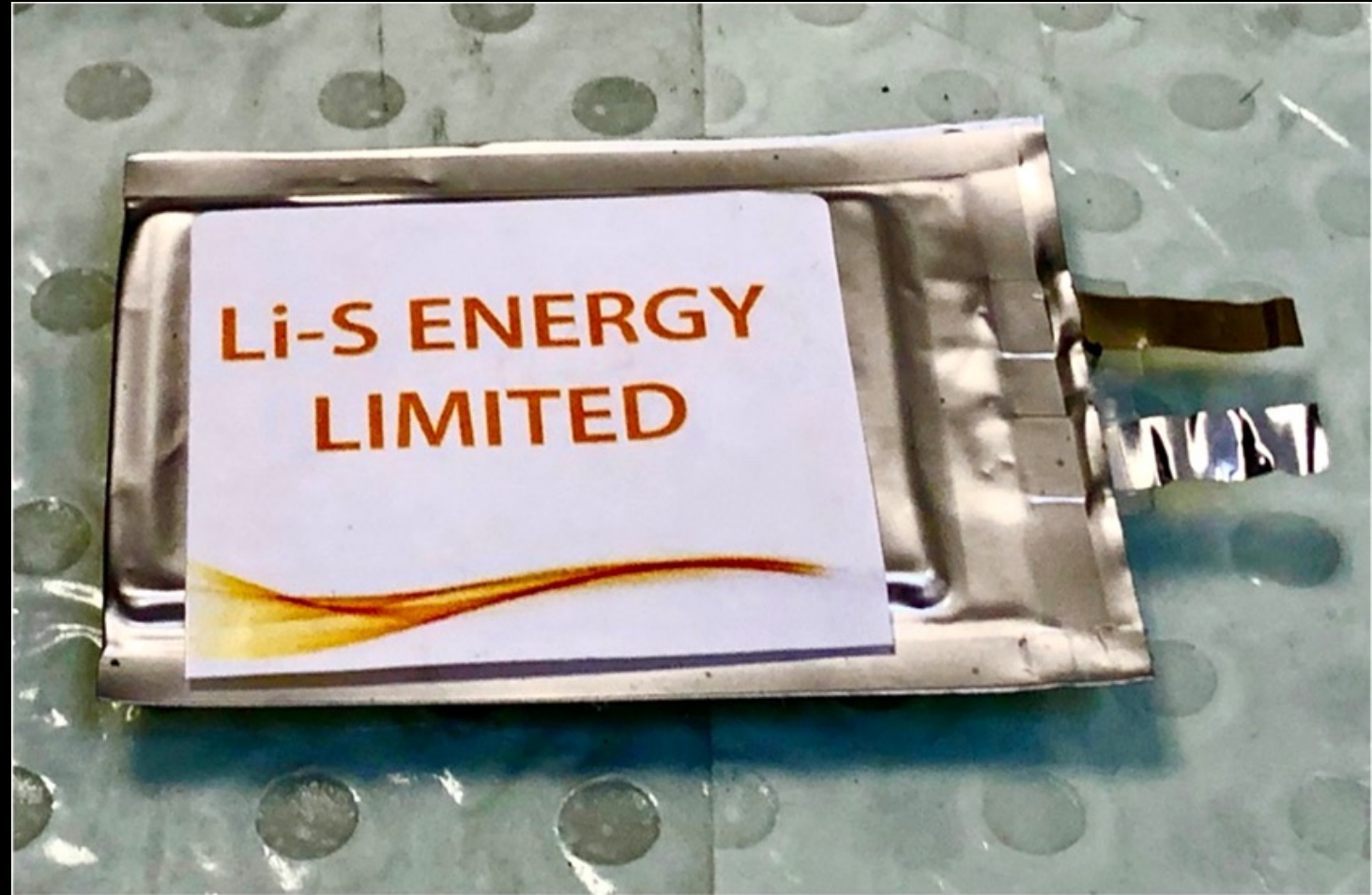
An Li-S Energy multi-layer lithium sulphur battery cell ready to start cycle testing
