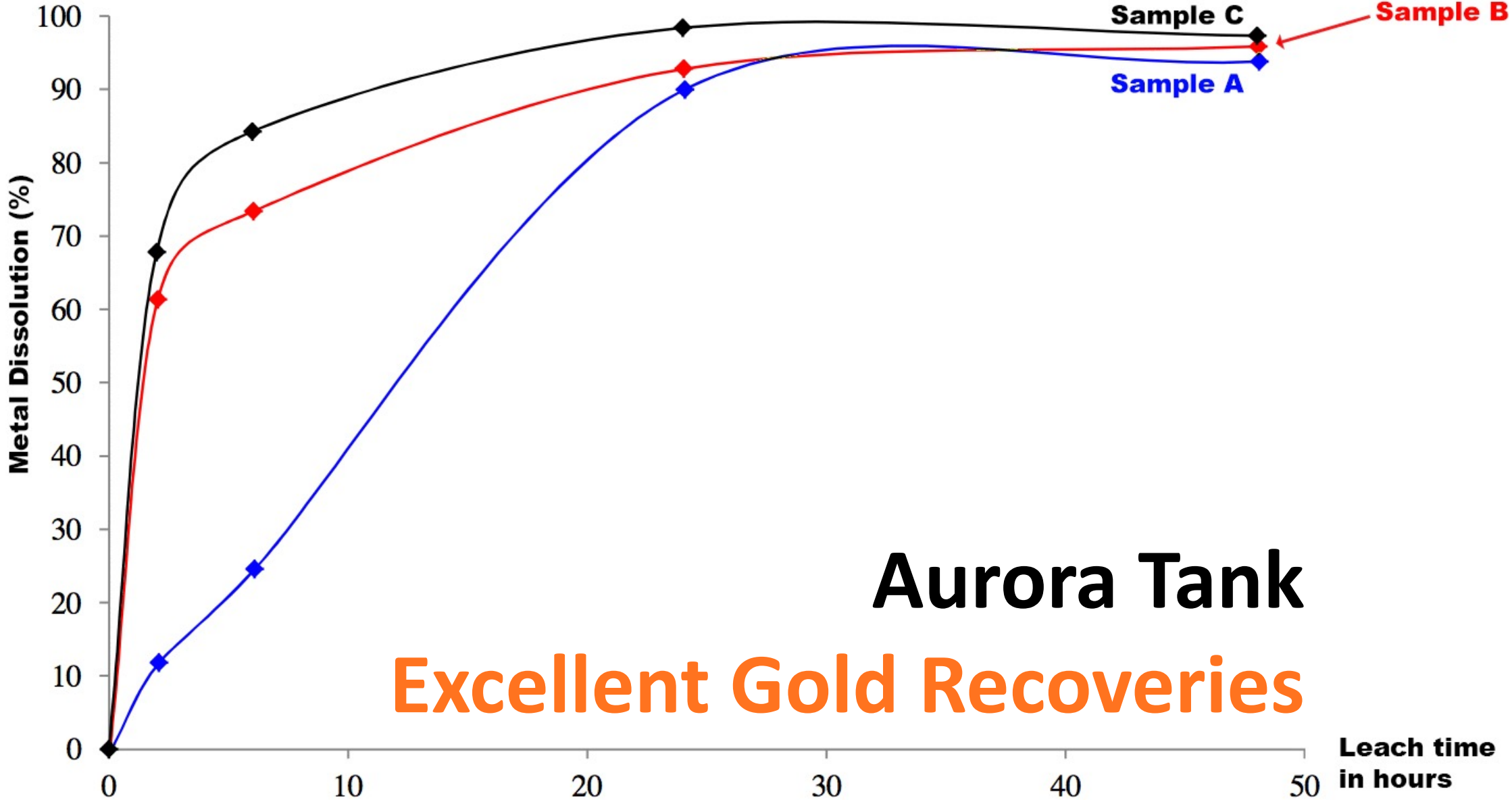
Gold Recoveries (in %) vs Leach times in hours (for the 3 test samples)
