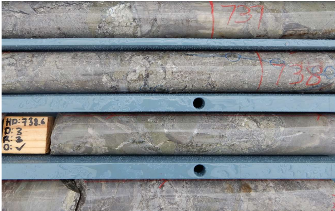
Fig 12 is a core photo (NQ Core) showing a section of pyritic clast supported breccia 737m-739m in hole 21CAEDD003 containing 4%-5% sulphur, 5%-10% pyrite.
