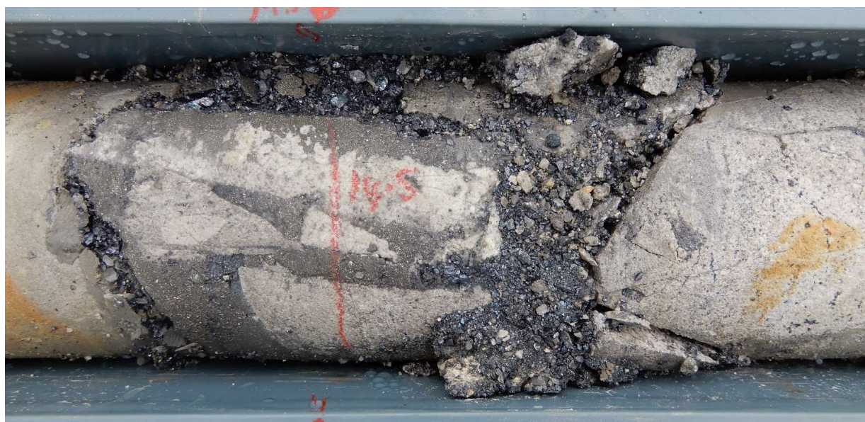
Fig 5 PQ Core photo hole 21CAEDD004, 14.5m. Chalcocite supergene zone replacing breccia infill of chalcopyrite and pyrite. 14.5m-15.0m assays 0.5m @ 1.70% Cu,0.28 g/t Au, 20.2 g/t Ag. 10% S.
