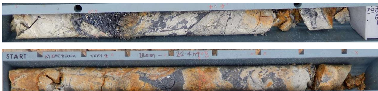
Fig 6 PQ Core photo hole 21CAEDD004, 19.5m-21m. Chalcocite supergene zone replacing breccia infill of chalcopyrite and pyrite. 19.5m-21.0m assays 1.5m @ 6.88% Cu,0.33 g/t Au, 18.1 g/t Ag. 10.3% S.
