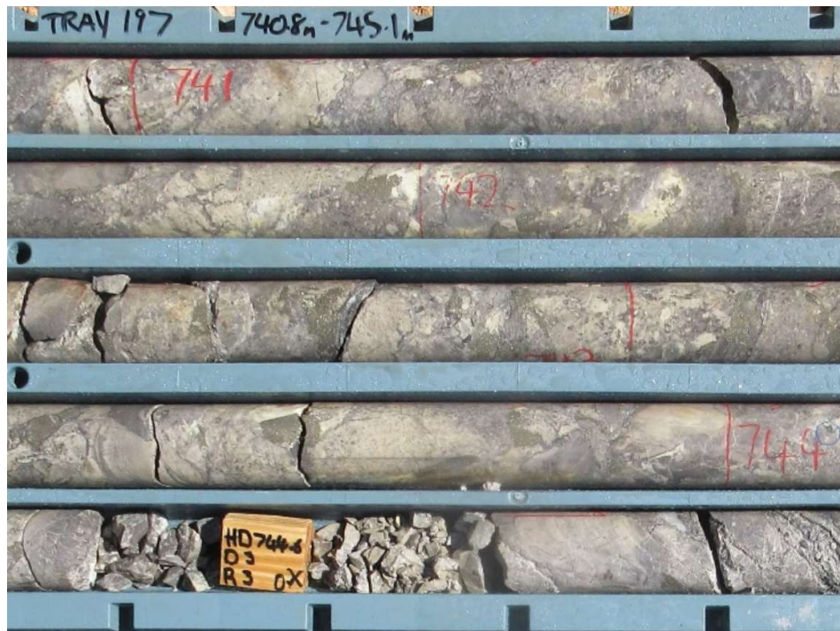
Fig 13 is a core photo (NQ Core) showing a section of pyritic clast supported breccia 741m-745m in hole 21CAEDD003 containing 4%-5% sulphur, 5%-10% pyrite.
