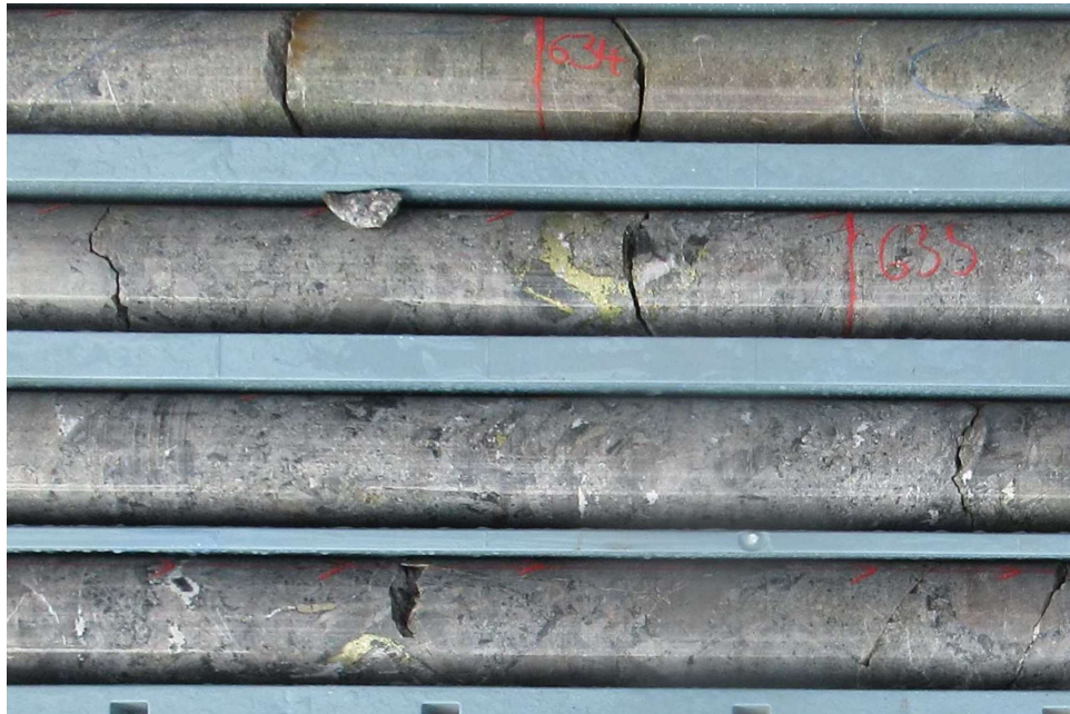
Fig 10 is a core photo (NQ Core) showing a section with chalcopyrite blebs in clast supported breccia 634m-636m in hole 21CAEDD003. Interval 634m to 635m contains visual estimate of 2% chalcopyrite, assay value of 0.82% Cu, 18.8 g/t Ag. 636m to 637m contains 0.23% Cu, 15 g/t Ag.
