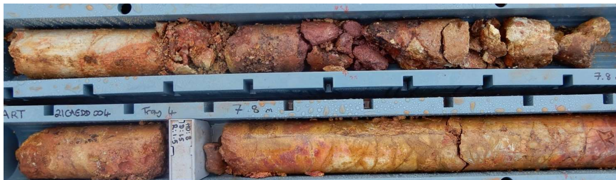
Fig 4 PQ Core photo hole 21CAEDD004, interval 7.0m-8.5m. Gossanous breccia , high oxidised sulphide content probably approximately originally 10%. 7.0m-8.0m assays 1m @ 0.78% Cu,3.4 g/t Au, 93 g/t Ag. (3 oz/t Ag).
