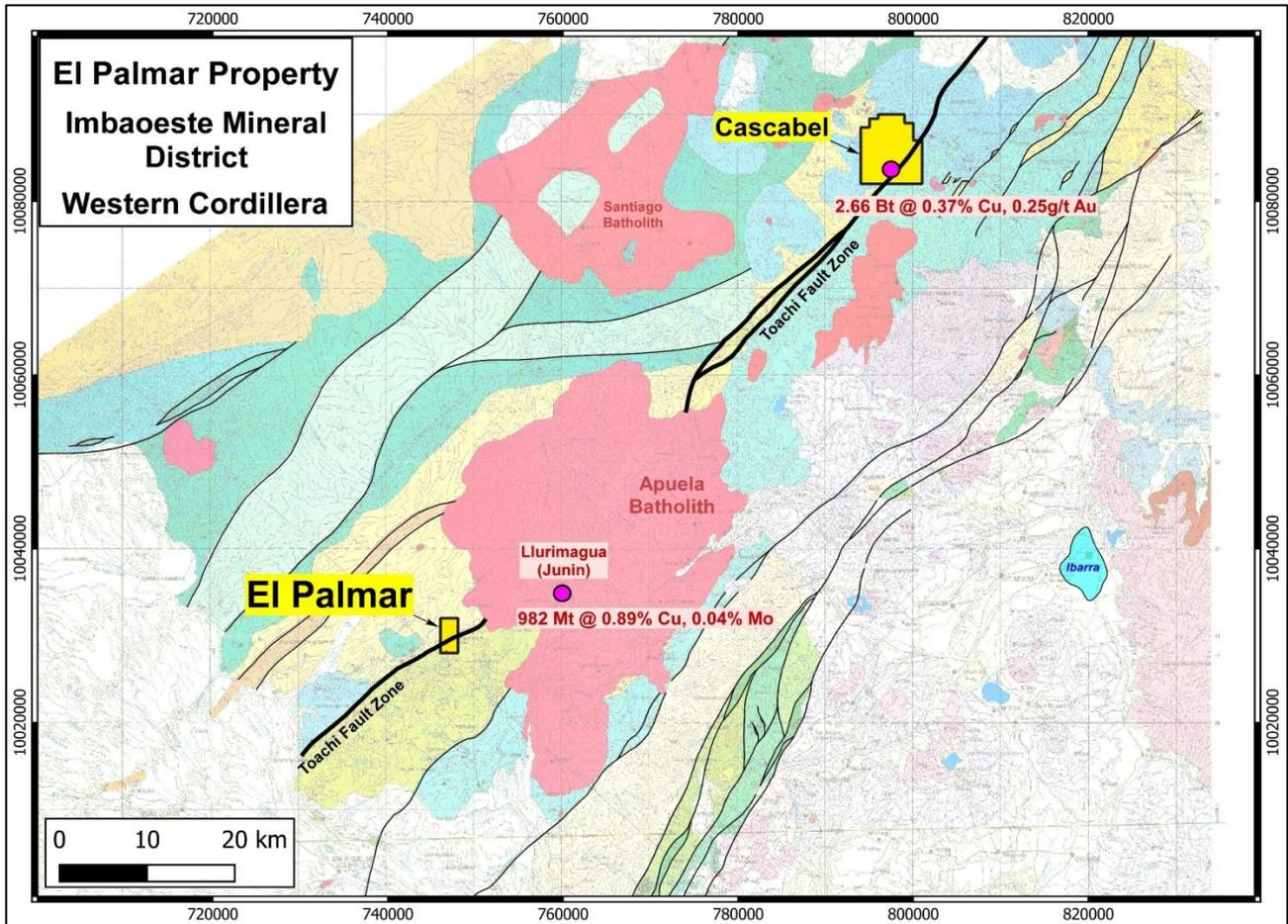
Figure 3: Location of the El Palmar project relative to the giant Lurimagua and Alpala (Cascabel) porphyry deposits, and the Toachi fault system.
