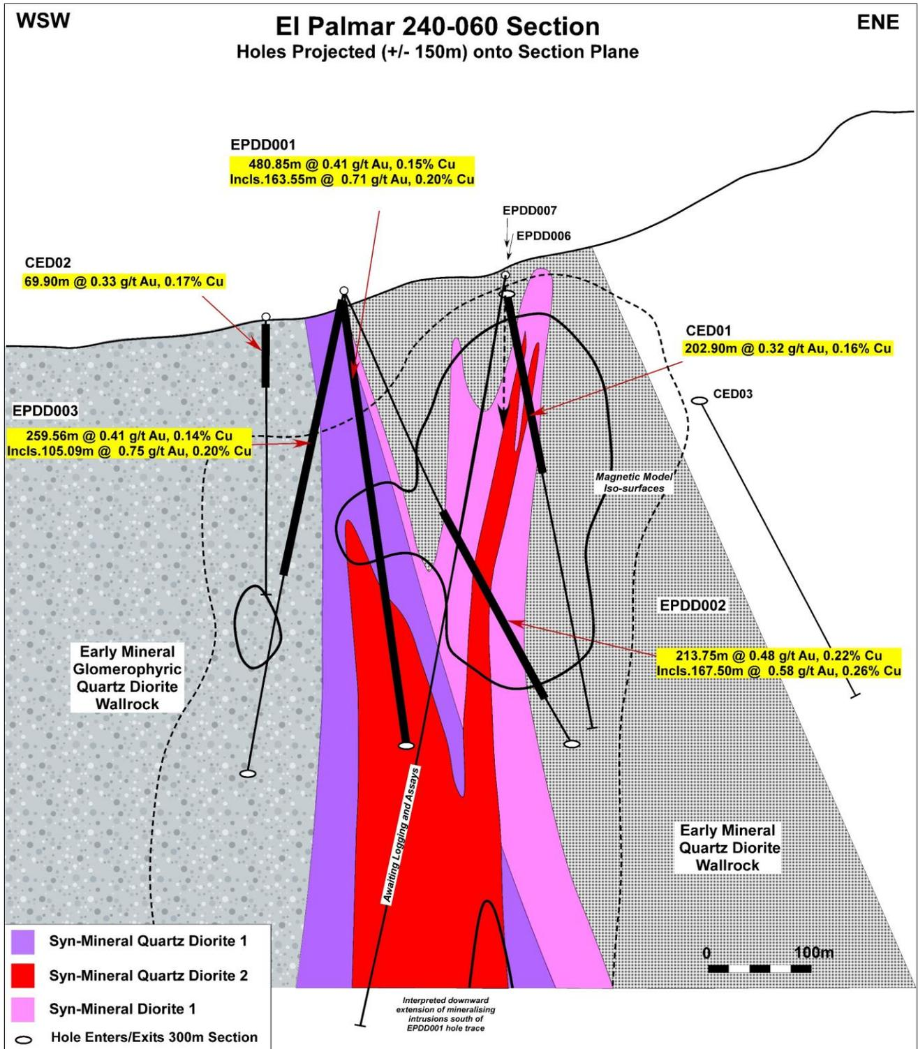
**Figure 2:** A composite cross section through EPDD001, 002, 003 and 006 at El Palmar, and showing the location of historical holes CED01, 02, 03. This section depicts the southeast side only of the larger El Palmar target area.
