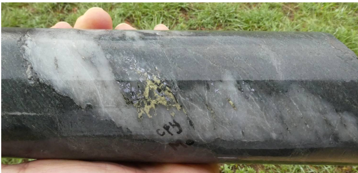
Figure 6. Deformed granular quartz vein with molybdenite along walls and internal chalcopyrite (BTDD004, 120.3m). Several such veins intersected in BTDD004 are interpreted as possible A or B Type veins within a porphyry system.
