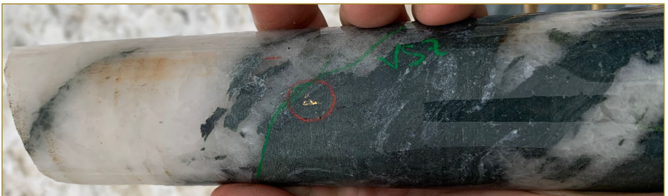
Figure 9: Photograph of coarse visible gold at the sheared vein margins in hole AUDD0229.
